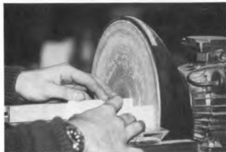
Fig. 13. A sanding wheel provides a quick alternative, but check its angle first!
