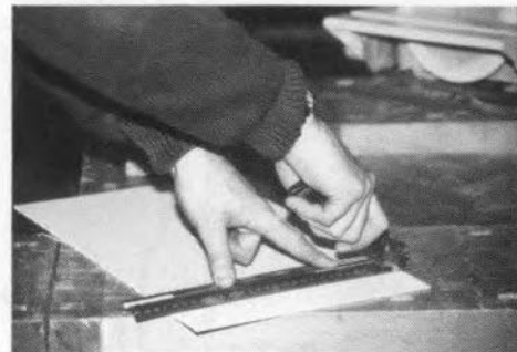
Fig. 4. Showing correct use of a safety ruler, scoring knife and the plastic sheet.
