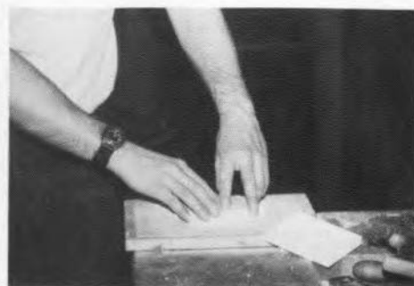
Fig. 22. Carefully sand the cut edges until they are free of saw marks.
