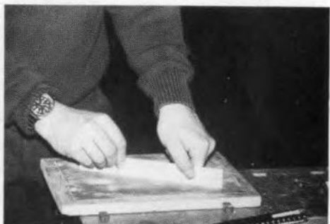
Fig. 8. Edges may be squared up on a sanding board with equal ease.
