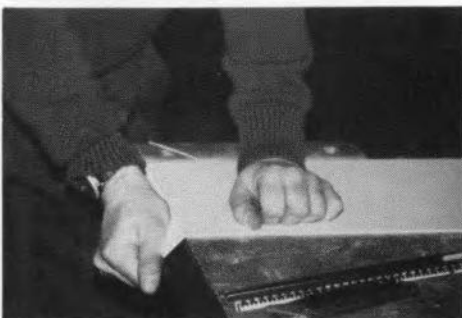
Fig. 5. Showing how to 'snap' the plastic cleanly over the edge of a bench.
