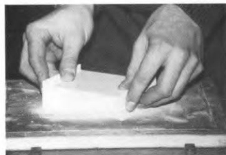
Fig. 15. Sanding the top of the box ready for the lid (shown upside down).
