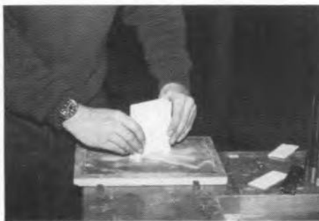
Fig. 12. Using a sanding board to square up the box ends.
