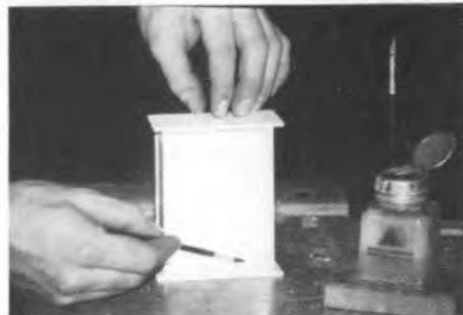
Fig. 14. Gluing the ends on to the box.
