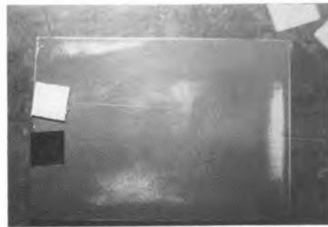
Fig. 35. Small patches showing through are not a problem — smooth finish is vital.
