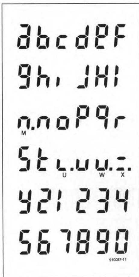
Fig.1. Representing letters and numerals on a 7-segment LED display.
