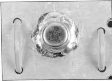
Fig. 4. Not for the faint-hearted: soldering the case of the MRF237 straight to the PCB ground plane.
