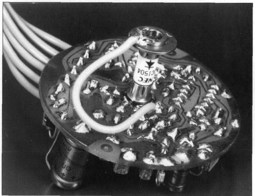
Fig. 1. Prototype of the radar detector, seen from the solder side of the PCB.
