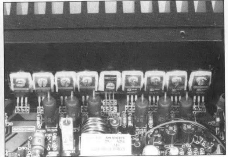
Fig. 8. The terminals of the driver, output and 'zener' transistors are bent as shown to make the devices protrude slightly from the board.
