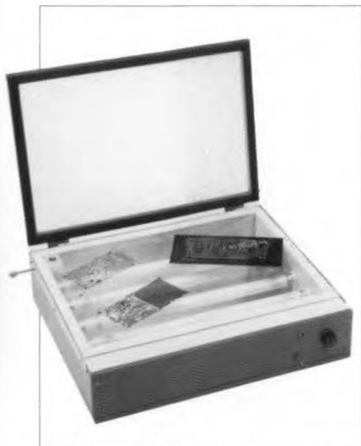
Fig. 1. Home-made UV exposure unit suitable for use with a vacuum pump for optimum contact between the photosensitive layer on the board and the emulsion on the film.
