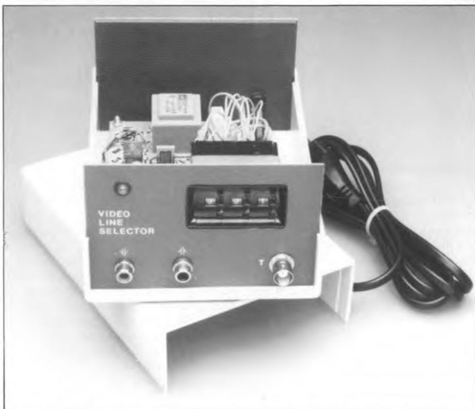
Prototype of the video line selector fitted in an ABS enclosure. BCD thumbwheel switches are fitted on the front panel for easy line setting. The video output socket (second from the left) enables the instrument to be hooked up in parallel with existing video connections.
