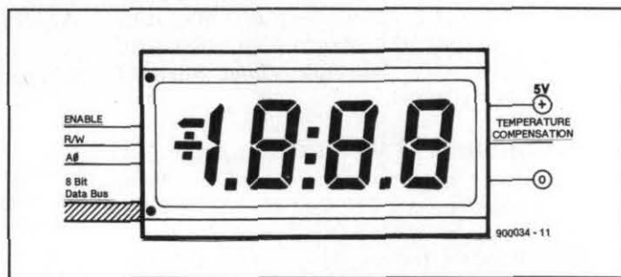
Fig. 1. Graphical representation of a 4-digit LCD module.
