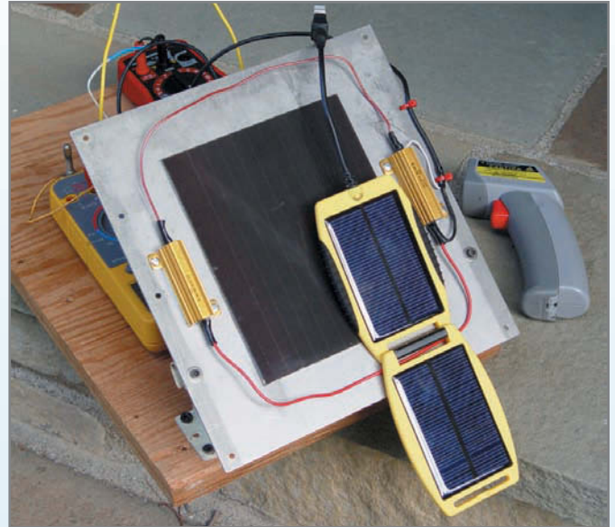
Photo 3 —I draped the Powermonkey solar panel over my test setup for full-sun measurements. Notice the lack of shadows due to a passing cloud: good for photography, bad for power!
