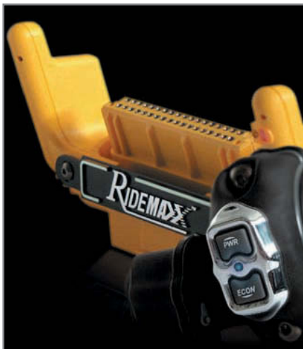
Photo 5—Embedded wireless has advanced to the point where it can make sense to use a radio to replace a single wire. The RideMaxx EFI controller uses a Bluetooth radio to connect the handlebar-mounted switch and under-the-seat controller.
