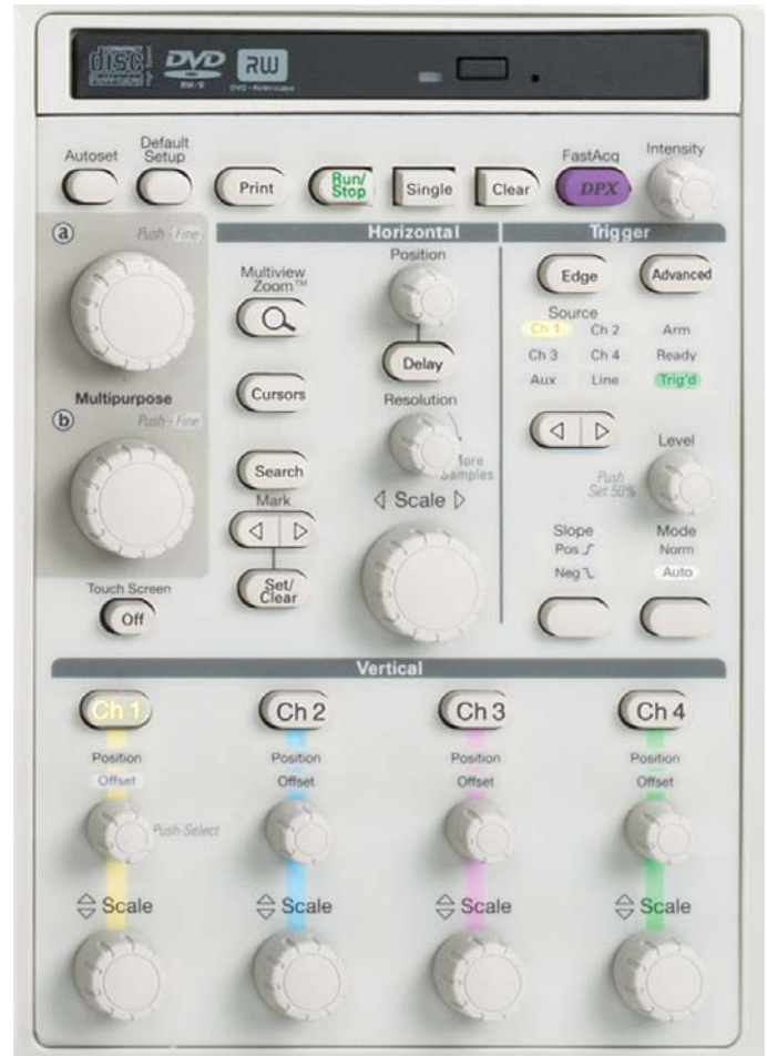
Figure 19. Front-panel control section of an oscilloscope.
