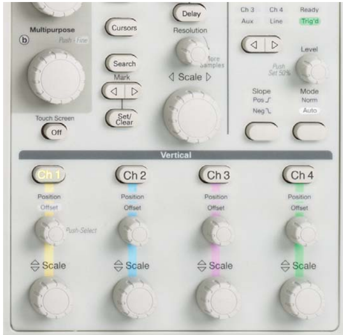
Figure 59. Traditional, analog-style knobs control position, scale, intensity, etc. – precisely as you would expect.
