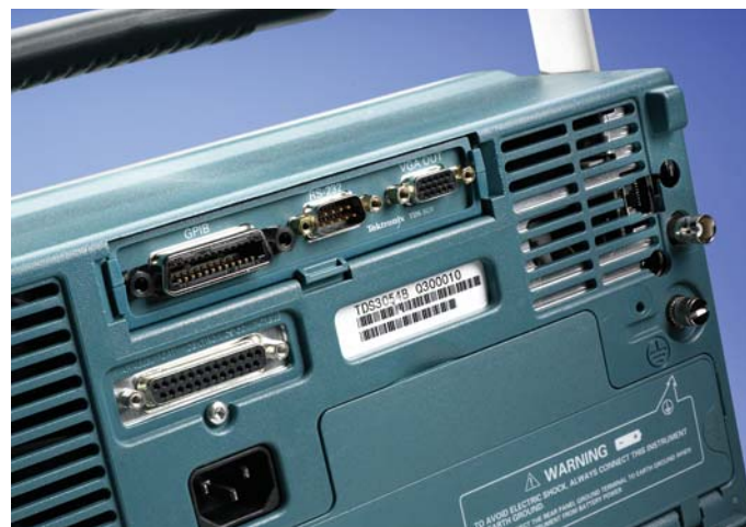
Figure 52. Today's oscilloscopes provide a wide array of communications interfaces, such as a standard Centronics port and optional Ethernet/RS-232, GPIB/RS-232, and VGA/RS-232 modules. There is even a USB port (not shown) on the front panel.
