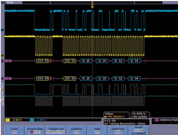
Figure 54. Serial bus analysis is accelerated with automated trigger, decode, and search on serial packet context.
