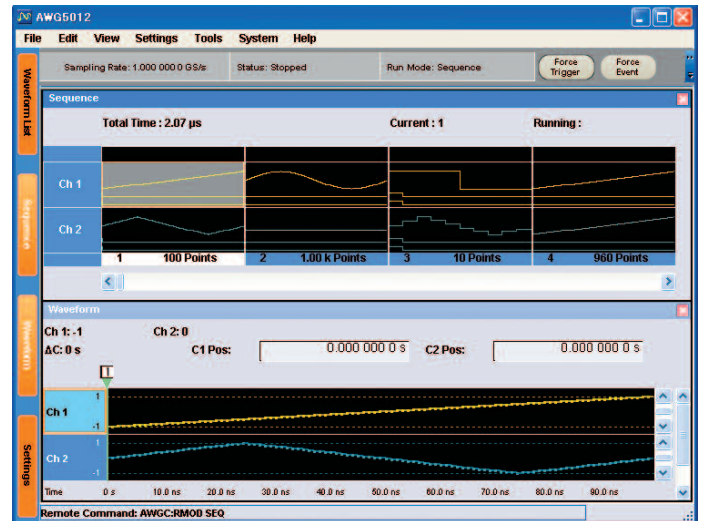
Figure 33. The Graphic editor and Sequence editor are combined for flexible waveform creation.
