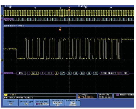
Figure 26. Triggering on Frame ID and Cycle Count, Searching through acquired data for Startup Frames.
