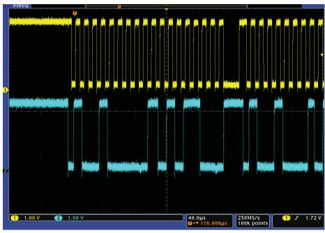
Figure 3. One message acquired from an I<sup>2</sup>C bus.
