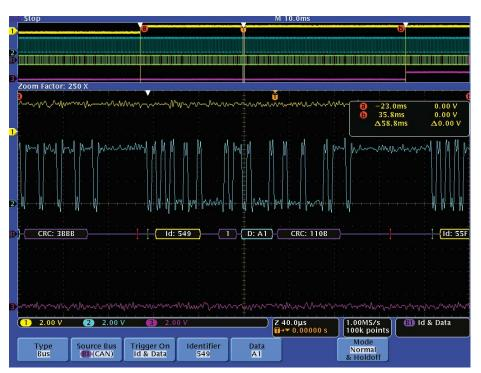
Figure 19. Triggering on specific identifier and Data on a CAN bus and decoding all messages in the acquisition.
