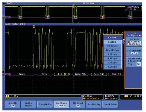
Figure 22. LIN bus setup menu and decoded frame.
