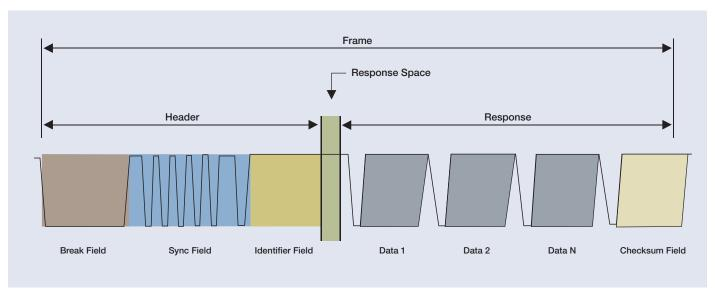
Figure 21. The structure of a LIN frame.
