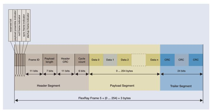
Figure 24. FlexRay frame structure.
