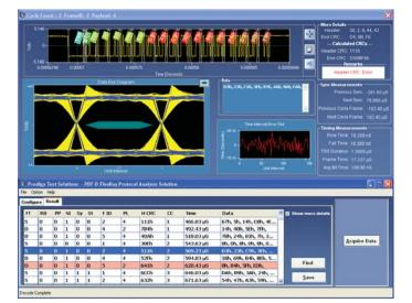
Figure 27. Eye Diagram analysis of a FlexRay signal.
