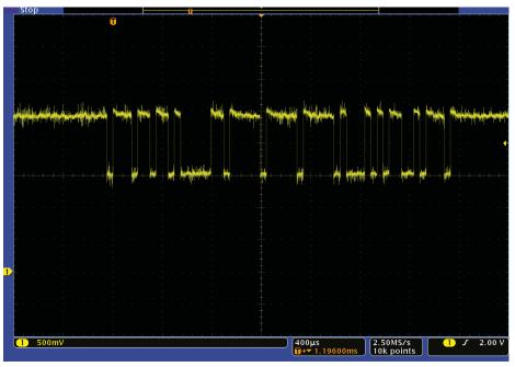
Figure 2. One message acquired from a CAN bus.
