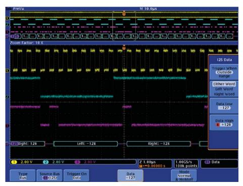
Figure 32. Triggering outside a range of values on an I<sup>2</sup>S bus.
