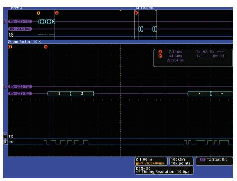
Figure 16. Measuring time delay between messages on two RS-232 buses.
