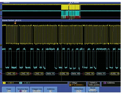
Figure 7. I<sup>2</sup>C address and data bus waveform decoding.
