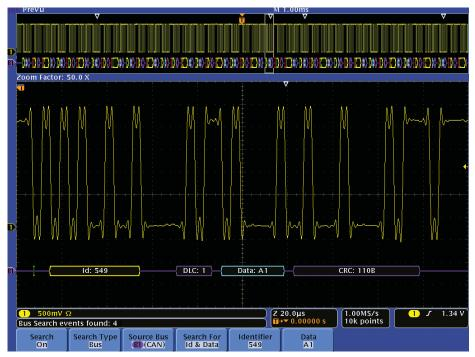
Figure 28. Searching on specified identifier and Data in a CAN bus aquisition.
