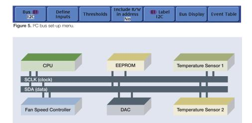
Figure 6. I<sup>2</sup>C bus example.
