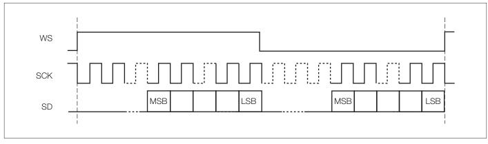
Figure 30 part III. RJ Format.
