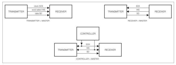
Figure 29. Different I<sup>2</sup>S bus configurations.
