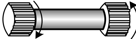
Figure 4-15 Barre de torsion
