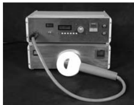
A pulsed field generator for magnetic stimulation.
