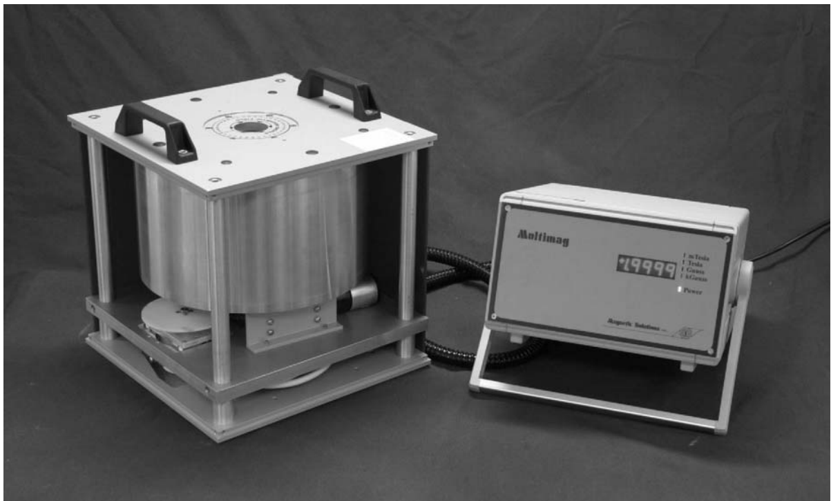
Figure 11 A 2.0 T permanent magnet flux source based on the structure of Fig. 10(a) (photo by courtesy of Magnetic Solutions Ltd).
