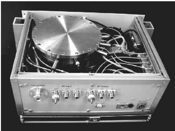
Figure 8 Commercial HTS subsystem for potential use in base stations. The filters and the LNA are inside a Dewar vacuum (left side), the metal cylinder in the right part of the assembly is the compressor of the Stirling-type refrigerator (from Kolesov et al. 2000).
