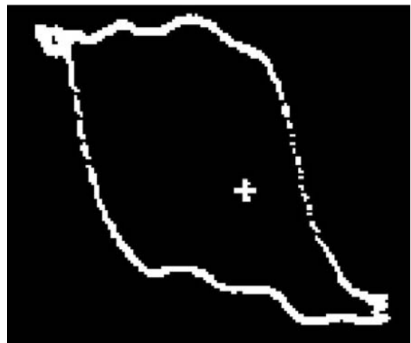
Figure 9 Measured resistance versus applied field R(H) for \text{Co}/\text{Al}_2\text{O}_3/80\text{NiFe} . The applied field is limited at \pm 1.6 \text{ kA m}^{-1} and the sample is initially saturated by + 3.2 \text{ kA m}^{-1} . Note that the MR hysteresis at zero field represents different magnetization combinations thereby yielding different magnetoresistances (after Wang and Nakamura 1995b).
