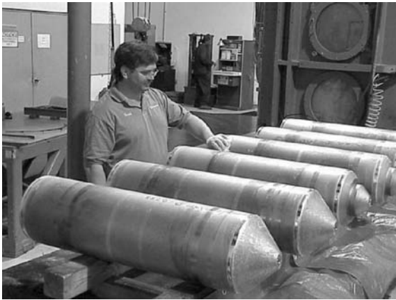
Figure 4 Monofilament Cu-clad Nb–Ti extrusion billets being inspected after welding (image courtesy of Hem Kanithi, Outokumpu Advanced Superconductors Inc.).
