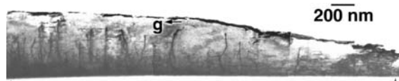
Figure 4 Cross-sectional transmission electron micrograph of a \text{YBa}_2\text{Cu}_3\text{O}_{7-\delta} film epitaxially grown on (100)\text{SrTiO}_3 by PLD showing \sim 10^9 threading dislocations \text{cm}^{-2} (reproduced by permission of Materials Research Society from J. Mater. Res. , 1990, 5 , 2620–32).
