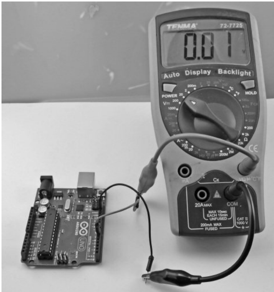
Figure 1-18 Measuring the output voltage
