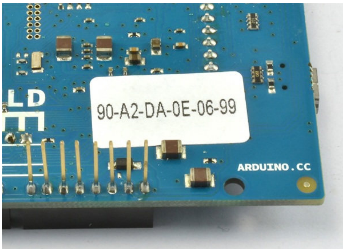
Figure 12-4 Mac address sticker on a WiFi Shield
