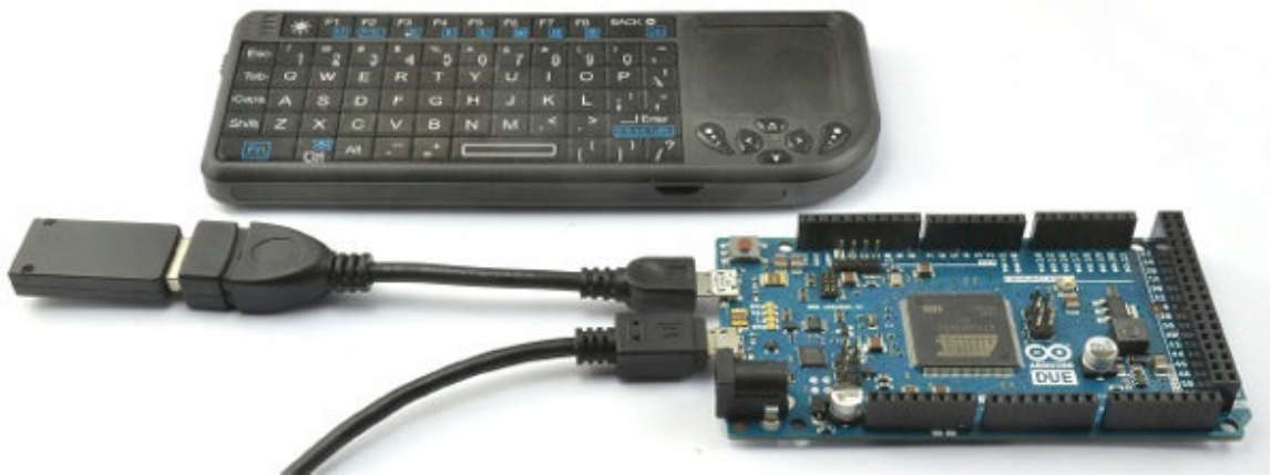
Figure 11-5 Arduino Due with a Micro USB OTG Host Cable and keyboard
