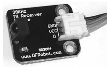
Figure 15-2: Pre-wired IR receiver module
