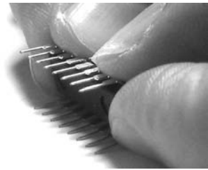
Figure 11-12: Bending the microcontroller pins
