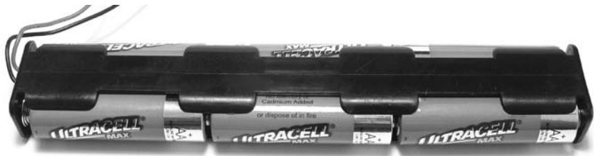
Figure 12-11: Battery holder with six AA cells
