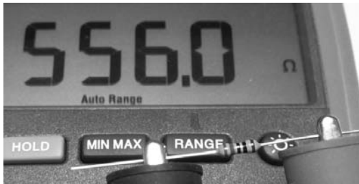
Figure 3-4: Multimeter measuring a 560-ohm 1 percent tolerance resistor
