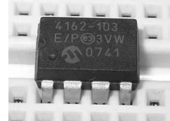
Figure 17-11: Microchip Technology's MCP4162 digital rheostat
