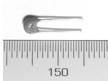
Figure 4-12: A 0.1 \mu\text{F} ceramic capacitor
