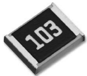
Figure 3-3: Example of a surface-mount resistor
