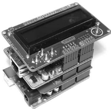
Figure 8-4: Three stacked shields with an Arduino Uno
