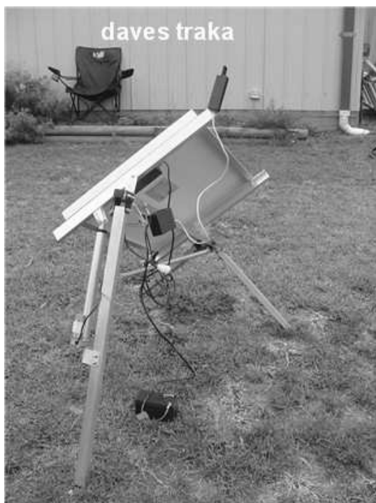
Figure 41. These 2 photos show the Solar Tracker built by J. Theismann. Note the fine workmanship on the mechanical details of the tracker assembly.
