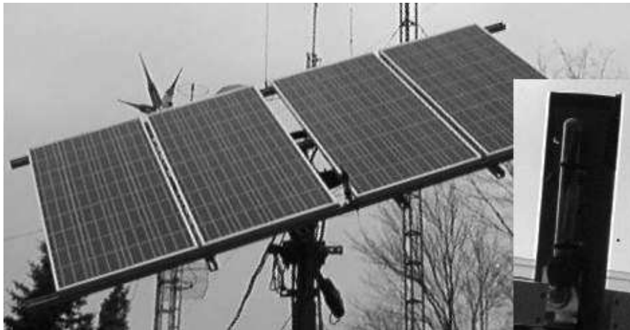
Figure 40. This Solar Tracker was built by Chuck in the Northeastern, U.S.A. Note the use of a linear DC actuator for the prime mover. The sun sensors are protected using an inverted test tube (photo insert).
