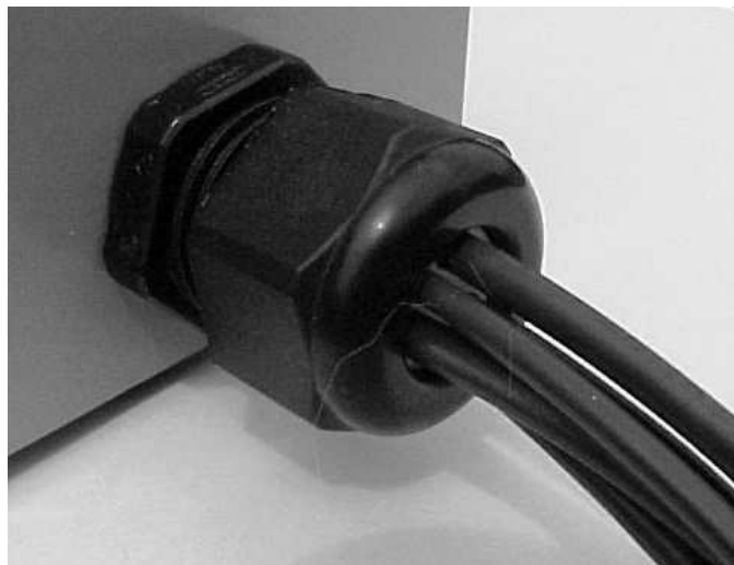
Figure 13. Example of wires exiting the box using a feed thru connector. This NPT feed through connector is McMaster-Carr part number #7807K43.
