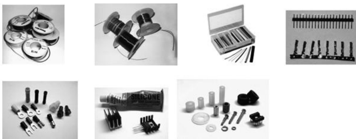
FIGURE 7.74 (a) Hookup wire. (b) Magnet wire. (c) Heat-shrinkable tubing. (d) 0.100-in. male headers and 0.156-in. female crimp sockets. (e) Butt connectors, ring, spade, crimp-on quick disconnects, wire nuts. (f) Heat sinks and heat sink compound. (g) Nylon and aluminum standoffs, washers, bolts, rubber feet, and IC socket.
