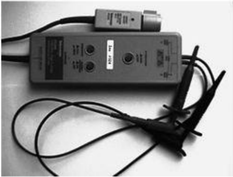
FIGURE 7.58 (a) General-purpose 1X/10X passive probe with assortment of probe attachments designed for use with a 1-M \Omega , 20-pF scope. At 1X, there is no attenuation, but the bandwidth is limited to between 4 and 34 MHz. At 10X, signals are reduced to one-tenth their original magnitude, while the bandwidth increases from between 60 and 300 MHz, depending on the probe and scope. (b) Active probe used primarily for high-frequency, low-voltage work. An active probe's internal FET provides extremely low-input capacitance (>1 pF) that allows for high bandwidths (500 MHz to 6 GHz) and minimal circuit loading. The probe typically comes with a 50- \Omega output impedance to drive a 50- \Omega cable, making it possible to increase probe cable length. It may require a special scope with a power connector/signal connector, or an external power source. A limited voltage range of \pm 40 V is typical. (c) Differential probe houses an internal differential amplifier that allows you to make differential measurements (between any two points, not just between one point and ground). Differential probes come in 50- \Omega and 1-M \Omega packages, and may require a special scope with a power connector/signal connector or an external power source. (d) High-voltage probe used for heavy-duty measurements of voltages over 2.5 kV. The P6015A from Tektronix can measure dc voltages up to 20 kV (RMS) and pulses up to 40 kV. It comes with a bandwidth of 75 MHz. Other high-voltage probes, often termed 100X, 1000X, will provide varying maximum voltage and bandwidth limits.
