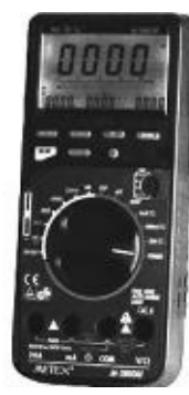
FIGURE 7.53 Left: HP 34401A bench DMM with 6.5-digit resolution and computer interface. Center: MetRex 3¾ digital DMM loaded with handy features, such as an RS232 interface, true RMS, temperature, inductance, capacitance, logic analyzer, transistor hFE tester, diode tester, and frequency counter. Right: A simple analog meter useful for monitoring trends.
