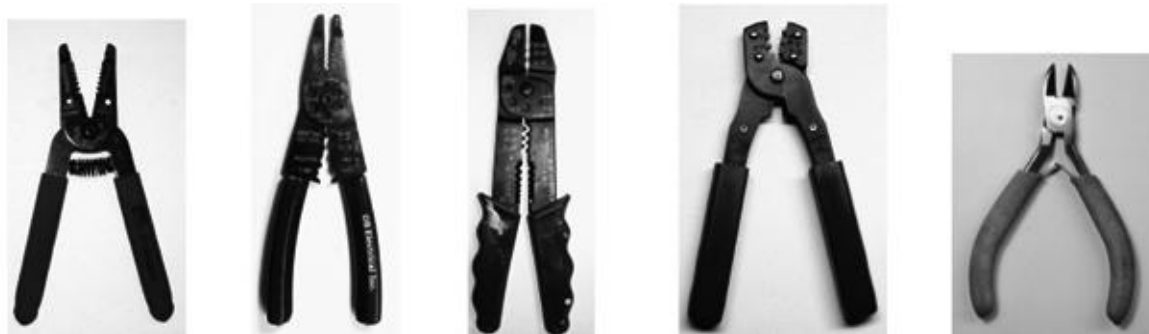
FIGURE 7.73 (a) Stripper (16–26 AWG). (b and c) Solderless crimping tools with additional features. (d) D-Sub crimping tool. (e) Diagonal cutter.
