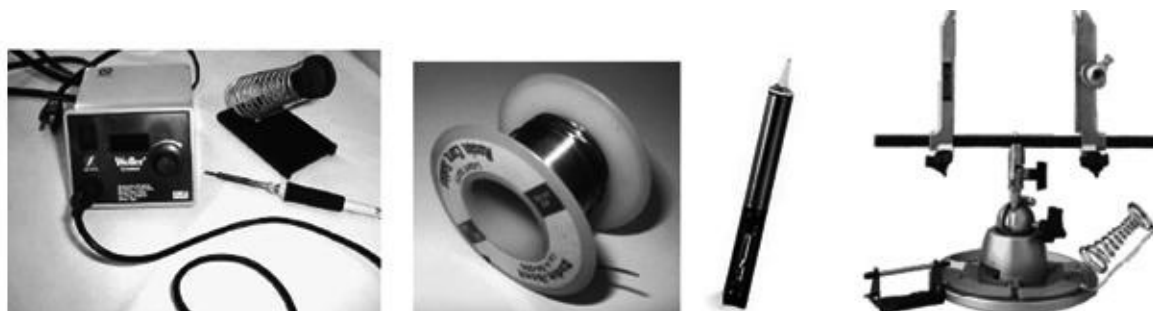
FIGURE 7.70 Various soldering items: temperature-controlled soldering iron with digital display of tip temperature, roll of 60/40 rosin-core solder wire, solder pump, PanaVise Electronic Work Center for holding circuit boards while soldering.
