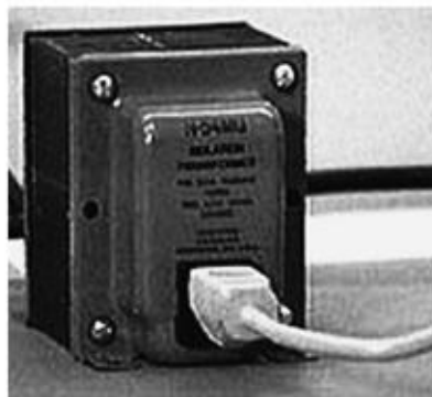
FIGURE 7.63 Basic schematic of a mains isolation transformer used to isolate the load from the source, as well as provide ground fault protection. An isolation transformer should be used whenever you work on nongrounded equipment with no input isolation, such as switch-mode power supplies. Notice that the voltage difference from secondary winding leads to earth ground is 0 V, unlike the 120-V difference in the primary side from hot to earth ground.
