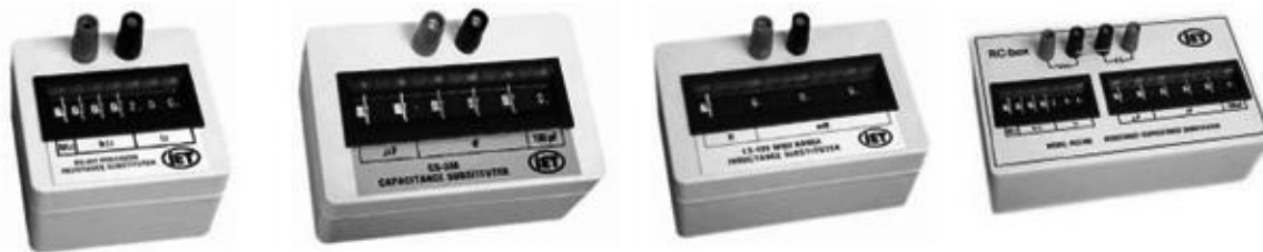
FIGURE 7.66 Selection of resistance, capacitance, inductance, and RC boxes from IET Labs, Inc. Resistance boxes come in seven- (0 to 9,999,999 \Omega , 1- \Omega resolution) and nine- (0 to 99,999,999.9 \Omega , 0.1- \Omega resolution) decade types. Capacitance boxes come in six (0 to 99.9999 \mu\text{F} , 100-pF resolution) decade types. Inductance boxes come in three (999 mH, 1-mH resolution) and four (9.999 mH, 1-mH resolution) decade types. RC boxes come with mixed decade selections given in provision R and C boxes. Uses thumbwheel switches to dial in resistance, capacitance, and inductance values. Accuracy is typically 1 percent or better.
