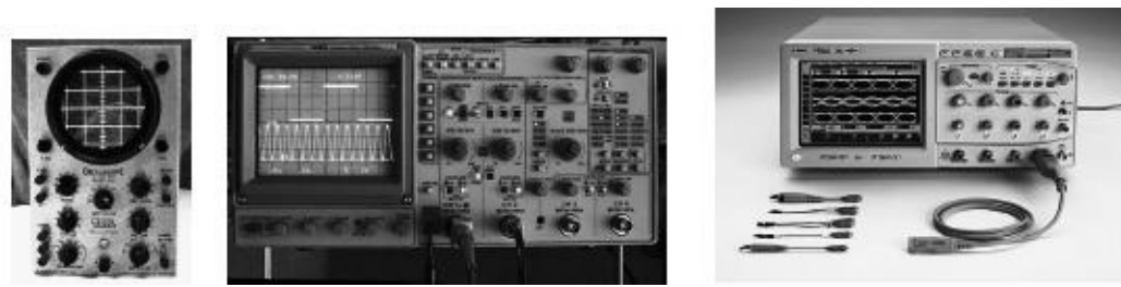
FIGURE 7.55 From vintage to high-tech, scopes will cost you accordingly. Left: An Eiko TR-410 10-MHz scope for around $30 on eBay. It's an incredibly slow scope by today's standards, but it's okay for general-purpose work on low-frequency circuits. Center: Tektronix 2246 100-MHz, four-channel analog oscilloscope with voltage and time cursors with on-screen readout. For about $400, used, on eBay, it's a good investment for general-purpose testing. Right: Cutting-edge Infiniium 54850 oscilloscope with InfiniiMax 1130 probes has a 6-GHz bandwidth with a 20-Gsa/s sample rate on all four of its channels. It comes with a user interface based on Microsoft Windows XP Pro, and supports CD-RW, dual-monitor, and third-party software. Don't expect to be able to buy one for personal use, unless you plan on robbing a bank. At the other end of the cost spectrum, new LCD-based scopes can be bought for around $55 (check out http://store.nkcelectronics.com/digital-storage-oscilloscope-very-low-cost.html ) and take up a lot less bench space than a vintage scope.
