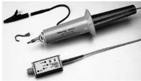
FIGURE 7.58 (a) General-purpose 1X/10X passive probe with assortment of probe attachments designed for use with a 1-M \Omega , 20-pF scope. At 1X, there is no attenuation, but the bandwidth is limited to between 4 and 34 MHz. At 10X, signals are reduced to one-tenth their original magnitude, while the bandwidth increases from between 60 and 300 MHz, depending on the probe and scope. (b) Active probe used primarily for high-frequency, low-voltage work. An active probe's internal FET provides extremely low-input capacitance (>1 pF) that allows for high bandwidths (500 MHz to 6 GHz) and minimal circuit loading. The probe typically comes with a 50- \Omega output impedance to drive a 50- \Omega cable, making it possible to increase probe cable length. It may require a special scope with a power connector/signal connector, or an external power source. A limited voltage range of \pm 40 V is typical. (c) Differential probe houses an internal differential amplifier that allows you to make differential measurements (between any two points, not just between one point and ground). Differential probes come in 50- \Omega and 1-M \Omega packages, and may require a special scope with a power connector/signal connector or an external power source. (d) High-voltage probe used for heavy-duty measurements of voltages over 2.5 kV. The P6015A from Tektronix can measure dc voltages up to 20 kV (RMS) and pulses up to 40 kV. It comes with a bandwidth of 75 MHz. Other high-voltage probes, often termed 100X, 1000X, will provide varying maximum voltage and bandwidth limits.
