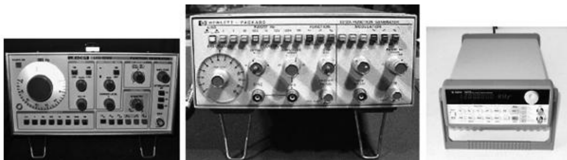
FIGURE 7.59 Left: Leader LFG-1300S, 2-MHz function generator with simple controls and many waveforms to select from, including amplitude modulation and linear/log sweep. Found for around $60, used, on eBay. Middle: HP 3312A function generator with a 0.1-Hz to 13-MHz bandwidth, providing sine, square, triangle, ramp, or variable symmetry pulses. Also has internal AM, FM, sweep, trigger, gate, or burst capability, along with external AM, FM, sweep, trigger, and gate capability. A great little instrument if you can find one for under $150. Right: Agilent 33120A 15-MHz function/arbitrary waveform generator, a high-performance signal source that provides sine, square, or triangular waveform signals over its 0.1- to 15-MHz frequency range. This instrument also provides a continuously variable dc offset and variable duty cycle, and the clock signal voltage levels adjusted to TTL components. It comes with both HPIB and RS-232 interfaces. Expect to pay around $500 for a used one.
