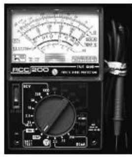
FIGURE 7.53 Left: HP 34401A bench DMM with 6.5-digit resolution and computer interface. Center: MetRex 3¾ digital DMM loaded with handy features, such as an RS232 interface, true RMS, temperature, inductance, capacitance, logic analyzer, transistor hFE tester, diode tester, and frequency counter. Right: A simple analog meter useful for monitoring trends.
