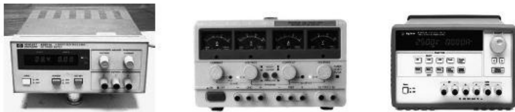
FIGURE 7.54 Constant current/voltage supplies with current lockout and voltage controls. The supply to the left comes with a negative, common, and positive terminal. The center supply houses three independent dc sources, two of which are variable, while the other is fixed at 5 V. The variable sections can be used independently, in series, or in parallel. To create a split supply, the two sections are placed in series, and the common becomes the junction between the two sections. The supply to the right houses split and fixed (5-V) sections. It can save and recall three voltage/current settings.
