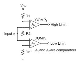
Figure 8.8: You can use a window comparator to identify analog signals that have exceeded a high or a low limit. You can accomplish this with two comparators, and by setting the threshold voltage with a voltage divider across the power supply. In this circuit, you will not require rail-to-rail input comparators.
