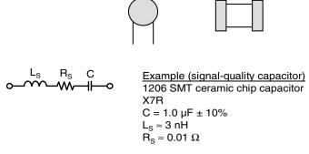
Figure 1.16: This illustrates a typical ceramic capacitor model. The parasitic elements of a standard capacitor is parallel resistance ( $R_s$ ), also know as effective series resistance (ESR), and series inductance ( $L_s$ ), also know as effective series impedance.
