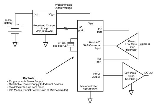
Figure 9.7: The lower-power, external-peripherals to the microcontroller only provide half of this battery-powered system implementation. The programmable capabilities of the microcontroller allow control of the power-supply voltage in the system (MCP1252-ADJ) and control of the microcontroller system clock and sleep modes.
