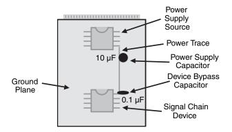
Figure 11.1: In analog and digital PCB design, you should place the bypass or decouple capacitors (0.1  $\mu$ F) as close to the device as possible. You should also place the power supply decoupling-capacitor (10  $\mu$ F) at the power-source or where the power-bus enters the board. In all cases, these capacitors should have short leads.
