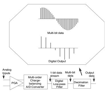
Figure 2.20: The purpose of a decimation filter is to slow down the output data rate in order to match the output data rate to the input frequency bandwidth. The FIR low-pass filter inputs a multibit data stream to the input of the decimation filter. The simplest decimation filter filters out several conversion results, while keeping enough to meet the output data rate of the converter.
