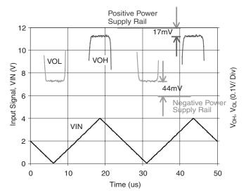
Figure 6.6: The bottom plot in this figure illustrates the input voltage swing to an amplifier that is configured in a gain of +2 V/V. The top plot shows the magnified output voltage of the amplifier. Included in the top portion of this plot is an indication where the positive supply rail is, with respect to  $V_{OH}$  and the negative supply rail with respect to  $V_{OL}$ .
