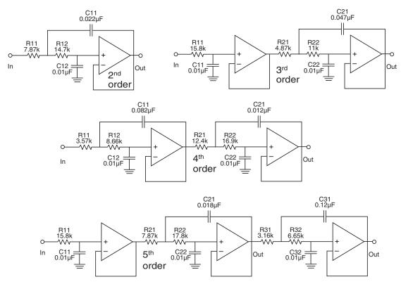
Figure 13.3: The design of the low-pass analog active filter is dependent on your selection of resistors and capacitors. You can design 1<sup>st</sup> order, 2<sup>nd</sup> order, 3<sup>rd</sup> order, 4<sup>th</sup> order, 5<sup>th</sup> order or higher. These are all Butterworth filters with a corner frequency or 1000 Hz and generated by a software filter program.
