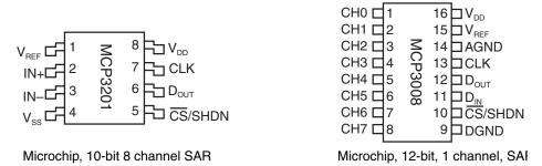
Figure 11.13: The SAR converter, regardless of resolution, usually has at least two ground connects; AGND ( $V_{ss}$ ) and DGND ( $V_{ss}$ ). The converters illustrated here are the MCP3008 and MCP3201 from Microchip.
