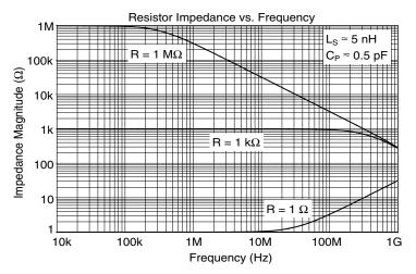
Figure 1.15: The impedance of a resistor changes from the defined DC resistance value to other values over frequency. The parasitic capacitance and impedance influence these changes.
