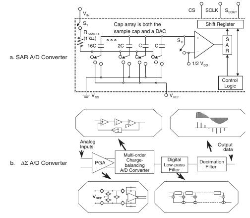
Figure 13.2: The (a) SAR analog-to-digital converter acquires high speed signals that only need minimal resolution. The (b)  $\Sigma$ - $\Delta$  analog-to-digital converter acquires a signal for higher resolution at slower speeds than the SAR converter.
