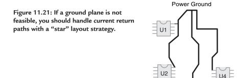
With this type of approach, the ground currents return to the power connection independently. You will note that in Figure 11.21 not all of the devices have their own return path. With U1 and U2, the return path is shared. This can be done if you use guidelines #4 and #5, following.
