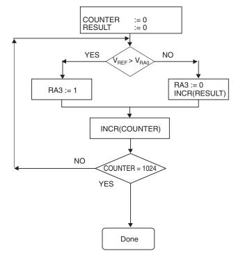
Figure 8.13: This is the sigma-delta A/D conversion flow chart, from the circuit shown in Figure 8.12. You should ensure that the cycle time through the flow chart is constant. This code runs until a conversion is complete.
