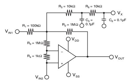
Figure 6.14: This circuit measures the DC parameters of Vos, Aol, CMRR and PSRR.
