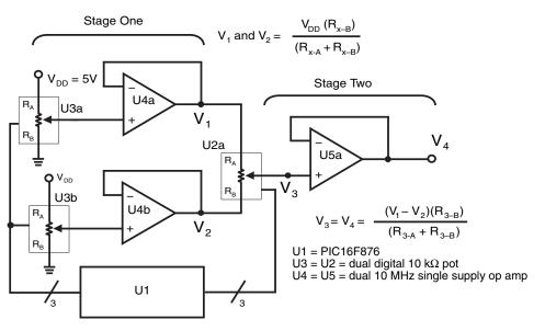
Figure 11.6: You can build a 16-bit DAC using three 8-bit digital potentiometers and three amplifiers to provide 65,536 different output voltages. If  $V_{DD}$  is 5 V in this system the resolution or LSB size of this DAC is 76.3  $\mu$ V.
