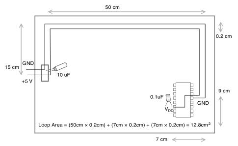
Figure 11.3: In this one layer board, the power trace and ground trace are laid next to each other on their way to the device on this board. Figure 11.2 shows a board where the traces are better matched. The opportunity for EMI into the electronics of this board is lessened by 679/12.8 or  $^{\sim}54x$ .
