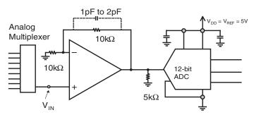
Figure 6.25: When the multiplexer switches from one channel to the next, it is possible that the amplifier receives a stepped signal. Figure 2.26 shows the step response of this amplifier circuit. The amplifier circuit does not make the system unstable. However, you should delay the A/D converter conversion while the op amp circuit is settling to final value.
