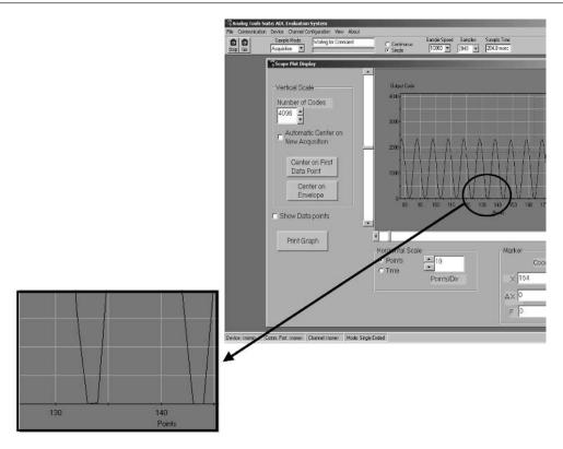
Figure 12.10: The time domain representation of the raw data from the FFT plot in Figure 12.8 shows that one of the amplifiers in the circuit is clipping the input signal on the negative rail. The sample rate of this test is 10 ksps. This graph has 2048 samples.
