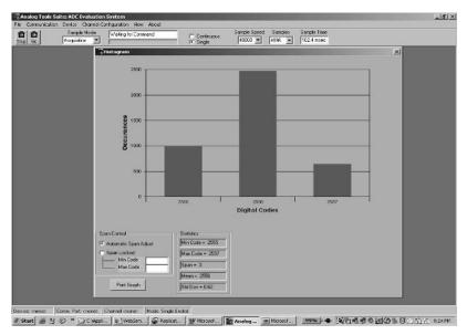
Figure 12.5: This is a collection of 4096 data outputs from the 12-bit A/D converter in Figure 12.1 The data rate of these 4096 data points is 40 ksps. From this histogram one could assume that the A/D converter or the analog signal path before the converter was noisy.
