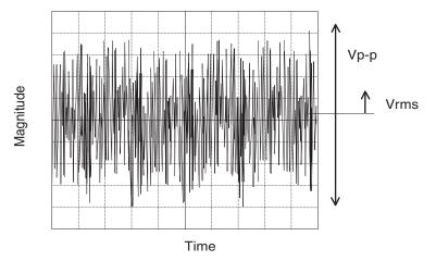
Figure 13.4: This is an oscilloscope picture of random noise. If your noise is gaussian, you can characterize and predict possible outcomes from your circuit by using statistics. The rms value of your sampled data is equivalent to one standard deviation.
