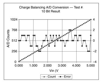
Figure 8.15: This graph shows the room temperature test data for the circuit shown in Figure 8.12 and a PIC16C623 microcontroller from Microchip. The input voltage range is 0.003 to 4.99 V. The maximum error found in the test was  $\pm 2$  counts. In this 10-bit system, the  $\pm 2$  LSBs is equivalent to  $\pm 9.8$  mV. The data from the A/D counts (left y-axis) was only one sample per point on the graph. Results may vary from part to part. V<sub>DD</sub> = 5 V.
