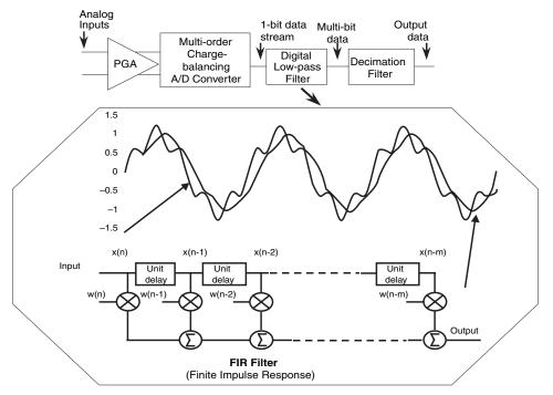
Figure 2.17: The filter illustrated in this diagram is a 1<sup>st</sup> order FIR filter. The digital low-pass filter of the  $\Sigma-\Delta$  converter further reduces the noise in the conversion process by averaging multiple digital codes in this rolling-averaging filter (FIR filter).
