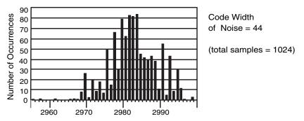
Figure 10.4: A 12-bit A/D converter is used to convert DC signal to hopefully one code. If you don't manage the passive (from resistors) and active (from amplifiers) noise well, the converter will give an unrepeatable result over time. The LSB size in this graph is 1.22 mV. The code width of forty-four codes equals 53.68 mV.
