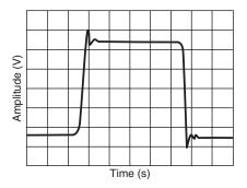
Figure 4.6: The step response of a 5<sup>th</sup> order, low-pass Butterworth filter has some ringing, but it eventually will settle after time. The amplitude of the ringing is dependent on the order (or number of poles) of the filter. The settling time is dependent on the filter's corner frequency and order. Generally speaking, the higher the order of the filter the higher the overshoot will be and the settling time will be longer.
