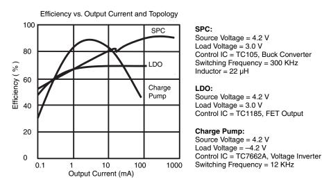
Figure 9.6: The graph illustrates the difference between the efficiency versus output current of SPC, LDO and charge pump circuits. This data demonstrates that the conditions of the specific system dictate the optimum solution.
