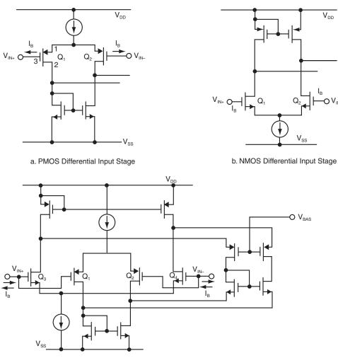
c. Composite PMOS and NMOS Differential Input Stage
