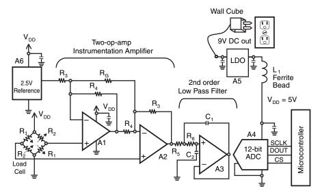
Figure 10.24: From Figure 10.3, this circuit has reduced resistors, lower noise amplifiers, a 2<sup>nd</sup> order low-pass filter, and an inductive choke or ferrite bead on the power supply. You can implement all of this tactics in the circuit to reduce analog noise and achieve 12-bit accuracy from the 12-bit ADC.
