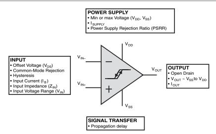
Figure 8.6: The comparator has the same basic input and output pins as the operational amplifier. There are several differences between the comparator and operational amplifier. The differences that the comparator has include a hysteresis in the input stage, propagation delay, and a digital output stage.
