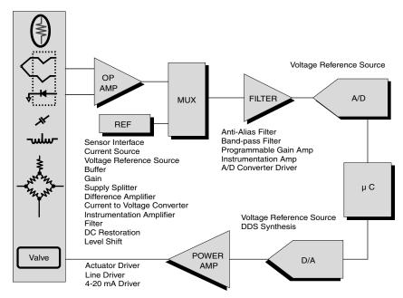
Figure 13.1: This diagram contains a classic sensor analog signal chain. There are a variety of sensors on the left side of this diagram. The amplifier stage conditions and the anti-aliasing circuit filters the sensor signal in preparation for the input of the ADC. The microcontroller device acquires that digital output code from the ADC.
