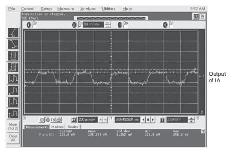
Figure 11.10: The 16-bit DAC in this new layout is showing a single code transition with no digital noise from the communication to the digital potentiometers.
