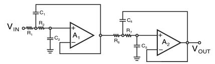
4th order (or 4-pole), low pass filter using two, 2-pole, Sallen-Key low pass filters
