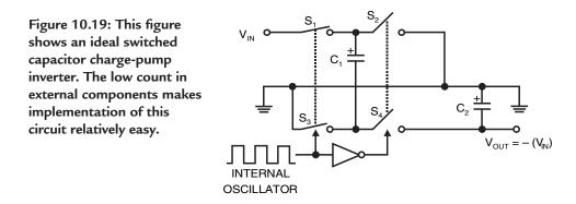
into the power trace, is device dependent. For details, refer to your vendor's data sheet. This device also emits noise due to the switching action through the capacitors.
