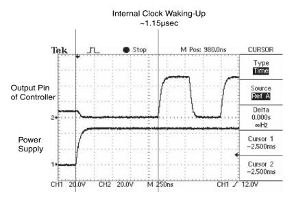
Figure 9.10: The start-up time of the internal clock is approximately 1.15  $\mu$ sec. This is considerably faster than the start-up time of the oscillator (in Figure 9.9).
