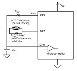
Figure 1.4: This circuit switches the voltage reference on and off at GP1 and GP2. In this manner, the time constant of the NTC thermistor in parallel with a standard resistor (RNTC || RPAR) and integrating capacitor ( $C_{INT}$ ) is compared to the time constant of the reference resistor ( $R_{REF}$ ) and integrating capacitor.
