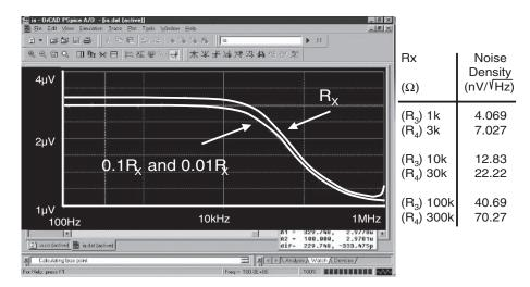
Figure 12.3: This SPICE simulation (also discussed in Chapter 10) suggests that the resistors in the circuit in Figure 12.1 cause noise. The resistors on the board were changed. Histogram test results verified this small improvement in the repeatability of this circuit.
