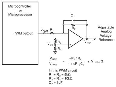
Figure 8.5: The 1<sup>st</sup> order filter uses an inverting amplifier configuration with an R/C pair in its feedback loop. This is an inverting amplifier circuit in a single-supply system. In this environment, you should reference the signal to halfway between  $V_{DD}$  and ground by using  $R_3$  and  $R_4$  in a voltage divider configuration.
