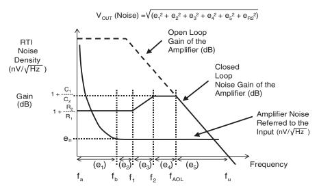
Figure 10.12: The noise of the amplifier is referred to the input of the device because the manufacturer doesn't know which configuration you are going to put your op amp into. With the referred-to-input values you can calculate your own referred-tooutput values, which you can use moving forward in the rest of your circuit.
