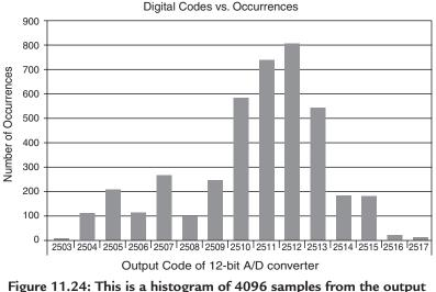
of the A/D converter. The PCB does not have a ground or power plane as shown in the PCB layout in Figure 11.25. The code of the noise from the circuit is 15 codes wide (Figure 11.23).
