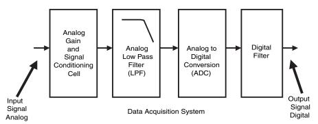
Figure 4.1: A data acquisition system will always require filtering in the signal path to remove unwanted signals. The analog filtering is required in order to get rid of higher frequency noise that is outside half of the sampling frequency of the converter. You use the digital filter to reduce lower in-band, frequency noise.
