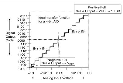
Figure 2.3: The transfer function of a 4-bit ADC bipolar analog input will produce a two's complement code as a digital output.
