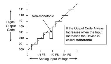
Figure A.6: This curve is nonmonotonic because an increase in the analog voltage can produce a smaller digital output code.
