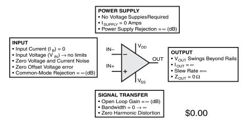
Figure 5.1: A perfect amplifier has an infinite input impedance, open-loop gain, power supply rejection ratio, common-mode rejection ratio, bandwidth, slew rate and output current. It also has zero offset voltage, input noise, output impedance, power dissipation and most importantly, zero cost.
