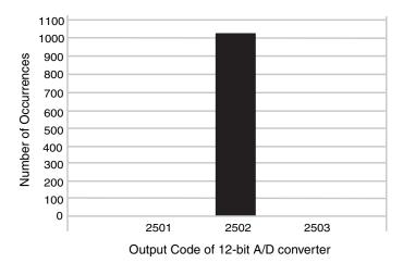
Figure 11.27: This diagram shows the conversion results of the circuit in Figure 11.22 plus a 2<sup>nd</sup> order, anti-aliasing filter. Additionally, the board layout includes a ground plane.
