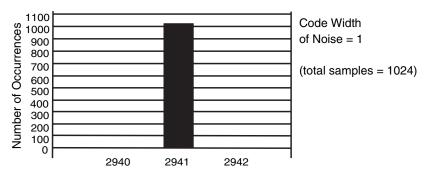
Figure 10.6: This data uses the same 12-bit A/D converter to convert DC signal to one code. In this new circuit, I am reducing the resistor values and using lower noise operational amplifiers. These two actions reduce the device noise in the circuit. An added ground plane reduces emitted noise. And finally, I add a low-pass filter, bypass capacitors, and a power supply inductive filter to reduce the conducted noise.
