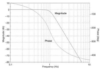
Figure 4.5: The frequency response of the Butterworth lowpass filter is maximally flat in the pass band. This plot shows the response of a  $5^{th}$  order Butterworth filter.
