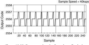
Figure 10.22: Power supply noise from the wall cube in Figure 10.3. The power supply frequency that appears at the output of the A/D Converter is approximately 2 kHz.
