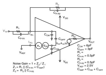
Figure 10.10: This amplifier circuit model is in an inverting gain configuration. This diagram illustrates the pertinent parasitics of the amplifier and resistors along with the calculation for noise gain.
