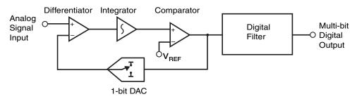
Figure 8.11: This is the modulator sigma-delta A/D converter. In the standalone sigma-delta A/D converter, the modulator, low-frequency noise moves out into higher frequencies. This 1<sup>st</sup> order modulator can achieve accurate conversions up to about 10-bits, without additional digital filtering.
