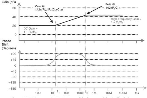
Figure 6.19: These are the Bode plots of the inverse of the feedback factor  $(1/\beta)$  for the circuit in Figure 6.18a using V<sub>STABILITY</sub> as the input source.
