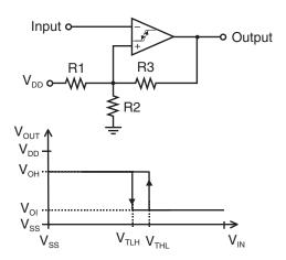
Figure 8.7: Using a feedback resistor, (R3) can enlarge the input hysteresis of a comparator, from the non-input to the output terminals. You use R1 and R2 to set a voltage reference for the comparator.
