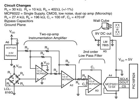
Figure 13.6: This is the analog portion of the block diagram drawing in Figure 13.5. The amplifiers and voltage reference tie into a microcontroller, PIC16F624 from Microchip. This portion of the circuit is powered from a 110 VAC to 9 VDC wall cube. The linear regulator, LM7805, converts the 9 V output of the wall cube to 5 VDC. (MCP1525, Microchip; MCP3201, Microchip)
