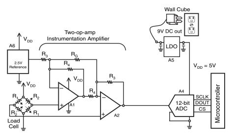
Figure 10.3: The two-op amp instrumentation amplifier gains the DC signal at the output of the load-cell sensor. The 12-bit A/D converter then digitizes that signal.
