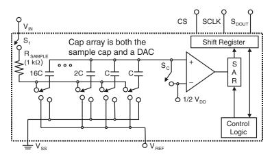
Figure 2.6: The modern day SAR converter uses a capacitive array at the analog input. This capacitive array and the remainder of the device are easily manufactured in CMOS, making it easy to integrate it with microcontrollers or microprocessors.
