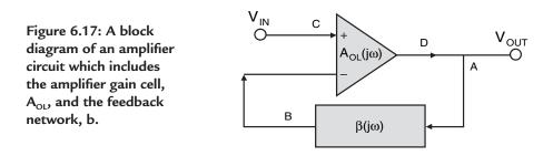
In Figure 6.17,  $\beta(j\omega)$  represents the feedback factor. Due to the fact that the open-loop gain of the amplifier (A<sub>OL</sub>) is relatively large and the feedback factor is relatively small, a fraction of the output voltage is fed back to the inverted input of the amplifier. This configuration sends
