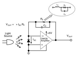
Figure 1.14: If you don't consider the parasitic capacitance of the feedback resistor, a transimpedance photosensing circuit can be unstable.
