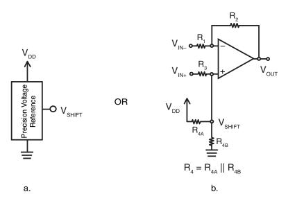
Figure 5.8: A precision voltage reference, (a) or a less expensive solution of replacing  $R_4$  of the voltage divider between the supply, (b) provides the voltage,  $V_{SHIFT}$ , of this difference amplifier.
