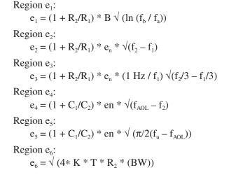
Note: In this calculation,  $C_1$  is the parallel combination of the input capacitors, or  $C_{P-R1} \parallel 2C_{CM} \parallel C_{DIFF} \mid C_2$  is the parallel combination of the feedback capacitors or  $C_{P-R2}$ .
