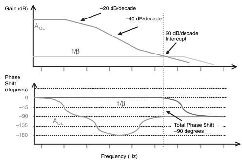
Figure 6.20: This closed-loop system is stable with a phase-shift of -90° at the intercept of the  $A_{OL}$  and  $1/\beta$  curves.
