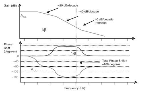
Figure 6.22: In a practical circuit implementation, given layout parasitics, this system is unstable.
