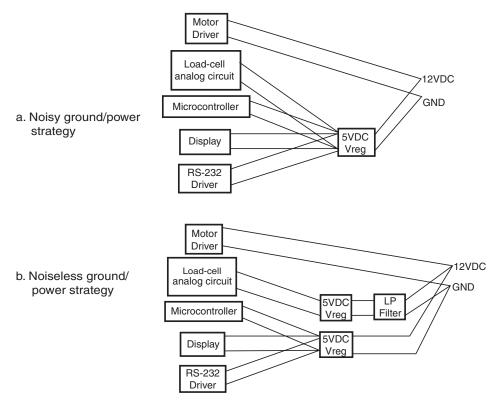
Figure 13.9: These are a few ground/power connection suggestions for the application circuit in Figure 13.5. The noise ground/power strategy (a) connects all 5 V systems to common power connections and the 12 volt noise driver (fan controller) to its own 12 V system. The conflict of the 5 V systems can cause circuit noise. Separation of analog and digital circuits will insure a lower noise environment.
