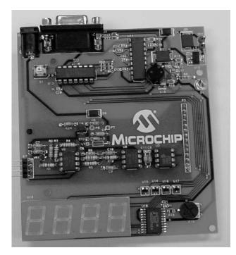
Figure 13.10: Combining analog and digital circuitry is easy if you keep track of your noise sources. The idea in this type of design is to keep noisy digital traces away from sensitive analog traces and devices.
