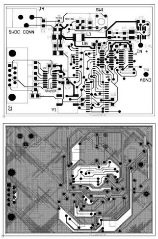
Figure 11.16: Bottom layer of an auto-routed layout of circuit diagram shown in Figure 11.17 and Figure 11.18.
