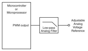
Figure 8.3: This is the hardware implementation of a PWM voltage reference using the controller or processor to generate the PWM signal. The analog low-pass filter changes the PWM signal to a DC voltage.
