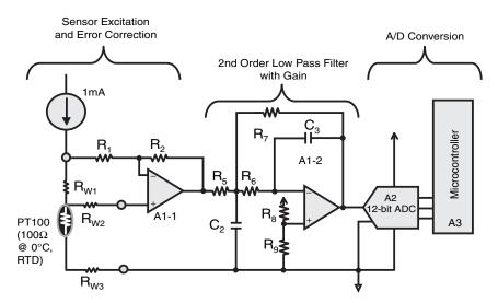
Figure 4.17: An RTD sensing circuit typically measures temperature at a low frequency rate. The anti-aliasing filter implemented in this circuit is 2<sup>nd</sup> order.
