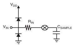
Figure 2.14: The input model of the sigma-delta converter is similar to the input model of the SAR converter. Consequently, if the external input impedance is too high, the offset and gain of a conversion can be compromised.
