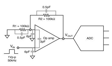
For example, the 100 k $\Omega$  resistor in the feedback loop of the amplifier will also have approximately a parallel 0.5 pF parasitic capacitor (see Figure 7.2). This parasitic capacitance on the breadboard to ground could be as high as 2 pF or 3 pF. If you use the amplifier's SPICE macromodel, with input impedances in the model and board parasitics, you will see this problem immediately in your simulation. If you breadboard the circuit, you most certainly will see this ringing.
