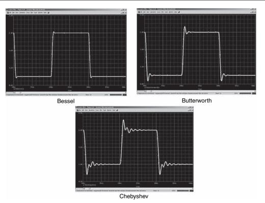
Figure 4.20: The time response of these three types of filters tell the tale when you are trying to decide which one to use in a multiplexed application circuit. I vote for the Bessel for the circuit in Figure 4.19.
