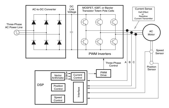
Figure 3.14: This is an AC motor control system configuration for three-phase control. The MOSFET, IGBT or bipolar transistor switches drive current through the AC motor. The "current sensors" sense this current. The ADC changes the signal from the current sensors into a digital code. The DSP engine then receives the digital code from the ADC. The DSP engine calculates appropriate PWM (pulse width modulator) instructions, again driving the totem pole power transistors into action.
