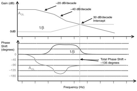
Figure 6.21: This system is marginally stable with a  $-135^{\circ}$  phase-shift at the intersection of the two gain curves.
