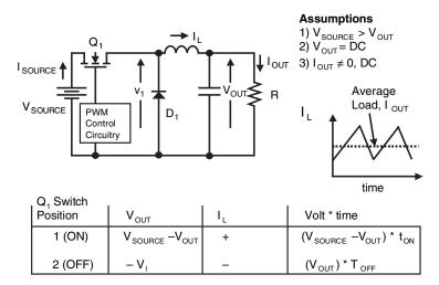
Figure 9.2: This illustration shows a Buck-SPC with the dynamic evaluation calculated for the device in the vontinuous mode. This power-supply solution is the most robust between a charge pump and LDO circuit.
