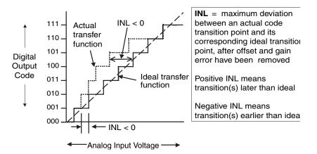
Figure A.5: INL is the aggregate of DNL errors and is equal to the maximum deviation for an ideal A/D converter transfer function.
