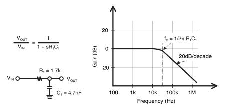
Figure 4.13: The passive, low-pass, analog filter uses a resistor and capacitor. The DC input and output impedance of this type of filter implementation is equal to  $R_1$ . The passive implementation is less expensive; however, the input and output resistance is high. As a result, this configuration usually needs one or two buffers.
