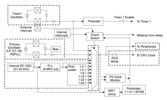
Figure 9.8: This diagram illustrates an example of three oscillator sources for a microcontroller. Externally, there are two clock connections (Timer1 and primary oscillator). Internally, there is another oscillator.
