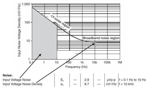
Figure 10.9: This is a representation of the noise of an example amplifier. The specifications for the noise performance of the amplifier are in tabular form at the bottom of this figure. These specifications numerically refer to the input noise voltage density versus frequency plot.
