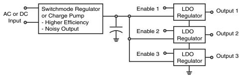
Figure 10.15: Power is taken from an AC (such as the wall) or DC (such as a battery) source and converted down (or up) to the required voltage level for the electronics. This conversion can be done in one stage or multiple stages, using LDO, switch-mode converters or capacitor charge pumps.
