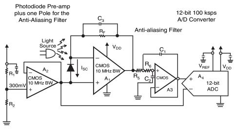
Figure 4.21: When light impinges on the photodiode, a charge is generated. This charge passes through the feedback resistor,  $R_{F}$ . The signal is then filtered with a 2<sup>nd</sup> order low-pass filter prior to the ADC.
