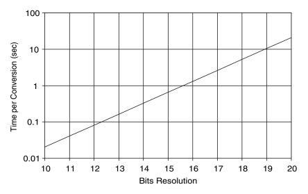
Figure 8.14: This graph shows the conversion time versus bits of resolution, assuming a 20 msec integration time while using the circuit shown in Figure 8.12.
