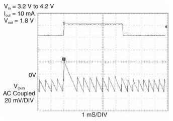
Figure 10.18: This figure shows the output voltage of a Buck-switch mode power supply converter with time. The converter is in its frequency mode of operation. The output signal produces a complex 20 mVp-p signal that has a switching frequency of 2000 Hz.
