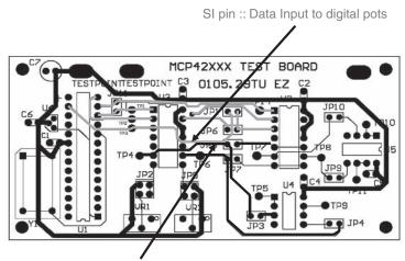
JP5 and Wiper out and amplifier input pins
