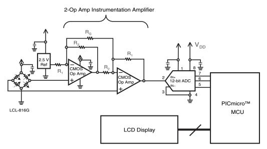
Figure 11.22: A two-op amp instrumentation amplifier, filtered and digitized with a 12-bit A/D converter, gains the signal at the output of the load-cell sensor. The result of each conversion is sent to the LCD display.
