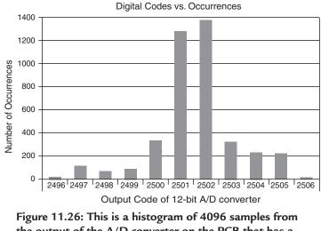
the output of the A/D converter on the PCB that has a ground plane as shown in the PCB layout in Figure 11.25. The code width of the noise is now 11 codes wide.
