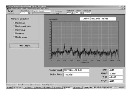
Figure 12.6: The FFT of the data shown in Figure 12.5 is a surprise. The histogram in Figure 12.5 uses the same data, but in a histogram representation instead of the FFT above. We expected random noise, which would look like a horizontal band across this graph. This data is actually showing that there is a signal with a fundamental frequency of approximately 1982.6 Hz. This data suggests that the once assumed "random" noise is anything but that.
