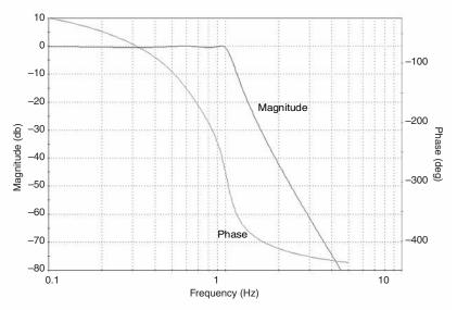
Figure 4.7: This is the frequency response of a  $5^{th}$  order, low-pass Chebyshev filter. This filter design has a 0.5 dB ripple in the pass band region. After the cut-off frequency, the attenuation of this filter is faster than the Butterworth or Bessel filter.
