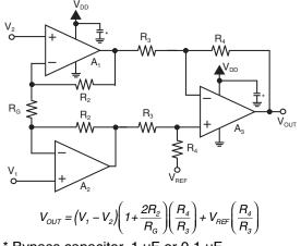
\* Bypass capacitor, 1  $\mu F$  or 0.1  $\mu F$
