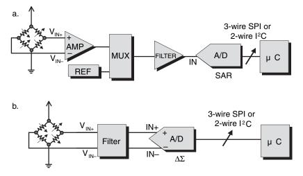
Figure 3.4: With many applications, you can use the SAR ADC or the sigma-delta ADC to digitize the analog signal. Many times the SAR ADC requires front-end analog gain circuitry. The sigma-delta ADC usually does not require this additional circuitry, but its slower speed will sometimes eliminate this type of device as an option.
