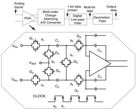
Figure 2.13: This switching network changes the analog input signal to a sampled voltage. This sampled voltage is taken in by the next stage where the signal is finally digitized into a one or zero.
