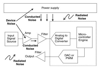
Figure 10.1: An analog application circuit can acquire noise from a variety of sources. You can categorize these noise sources into three groups: device noise, radiated noise, and conducted noise.
