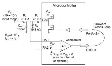
Figure 8.17: Configuration of the microcontroller for a sigma-delta conversion with a 10 V to 15 V range centered around 12.5 V.
