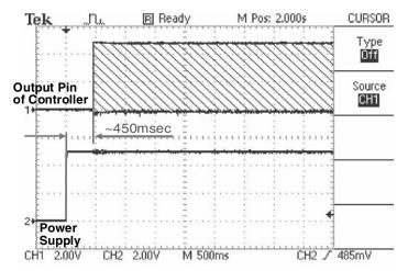
Figure 9.9: The clock connected to the controller is a 4 MHz crystal. In this oscilloscope plot, Channel 1 is a microcontroller output pin. The programming of the microcontroller toggles this output- pin every 12 instruction cycles. Channel 2 shows the power-supply to the controller,  $V_{DD}$ . The external clock to the controller becomes active approximately 450 msecs after power supply start-up.
