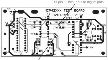
Wiper out and amplifier input pins
