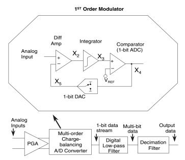
Figure 2.15: The multiorder charge-balancing stage of the  $\Sigma$ - $\Delta$  converter samples the input signal from the PGA stage and converts that signal to a one or a zero. Since this stage has a DAC in the feedback loop, the noise in this conversion is pushed out of the lower frequency band. This phenomenon provides the first step to an extremely low-noise conversion.
