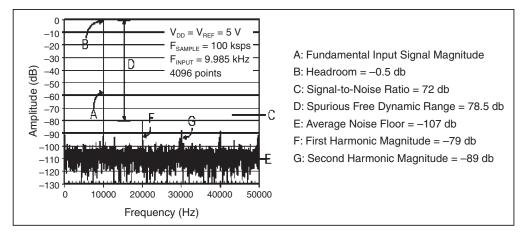
Figure B.2: Basic elements of the FFT plot include the fundamental input signal (A), signal headroom (B), signal-to-noise ratio (C), spurious-free dynamic range (D) and the average noise floor (E).
