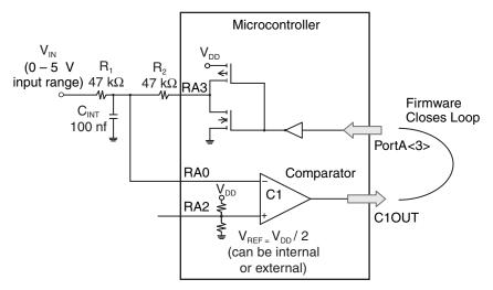
Figure 8.12: If a microcontroller has an internal comparator and timer, you can build a sigma-delta converter with two additional external resistors and one capacitor. In this configuration, a low-pass filter is a by-product of the external resistors and capacitor input network.
