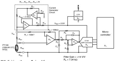
Figure 3.7: A SAR ADC digitizes the small signal from a three-terminal, RTD temperature sensor as long as an amplifier circuit gains this small signal from the RTD. In this circuit, the operational amplifier,  $A_4$ , is used to implement a gain as well as a  $2^{nd}$  order low-pass filter.
