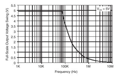
Figure C.3: The full power bandwidth of this amplifier is approximately 75 kHz.
