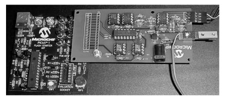
Figure 13.7: This figure shows the layout for the circuit in Figure 13.6. Although this figure does not show the backside of this board, there is a complete, uninterrupted ground plane on that side.
