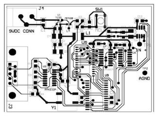
Figure 11.20: Bottom layer of a manual routed layout of the circuit diagram shown in Figure 11.17 and Figure 11.18.
