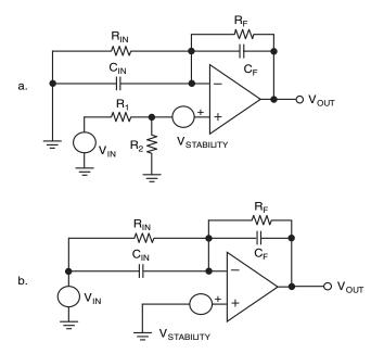
Figure 6.18: The input signal in circuit (a) at DC will be gained by  $(R_2/(R_1 + R_2)(1 + R_F/R_{IN}))$ . The input signal in circuit (b) has a DC gain of  $-R_F/R_{IN}$ . Neither of these gain equations match the DC gain of the feedback factor,  $1/\beta$ .
