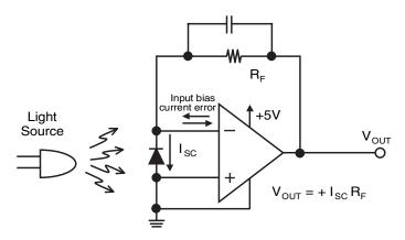
Figure 7.8: An amplifier with a low-input bias current in a transient-impedance amplifier circuit, like this one, is critical if you want to preserve reasonable accuracy. For this reason, CMOS or FET input amplifiers are preferred. If you try to simulate this circuit without the proper input bias current values, you will see an output voltage error at  $V_{out}$ .
