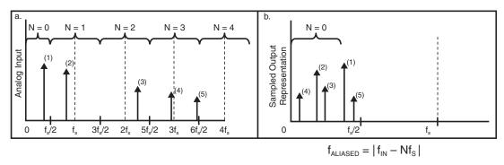
Figure 4.11: A system that is sampling frequency at  $f_s$  (a) will identify signals with frequencies below  $f_s/2$  as well as above. Input signals below  $f_s/2$  will be reliably digitized while signals above  $f_s/2$  will be folded back (b) and appear as lower frequencies in the digital output.
