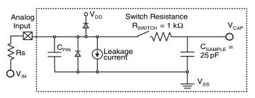
Figure 2.9: The combination of the external input resistance ( $R_s$ ) and internal switch resistance ( $R_{SWITCH}$ ) and the sample capacitor ( $C_{SAMPLE}$ ) form a low-pass filter that has a rise time. If an accurate conversion is desired, the external input resistance should be minimized or the sampling time of the converter should be lengthened.
