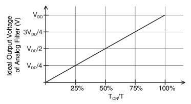
Figure 8.2: If a PWM signal is sent to an output port of the microcontroller and then through an analog low-pass filter, the output voltage of the filter with respect to  $V_{DD}$  is ratio matched to the ON time  $(T_{ON}/T)$  of the PWM signal.
