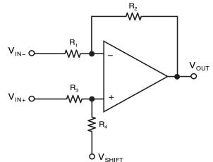
This circuit configuration will reliably take the difference of two signals as long as the signal-source impedances are low. If the signal source impedances are high with respect to  $R_1$ , there will be a signal loss due to the voltage divider action between the source and the input resistors to the difference amplifier. Additionally, errors can occur if the two signal source impedances are mismatched. With this circuit, it is possible to have gains equal to or higher than one.
