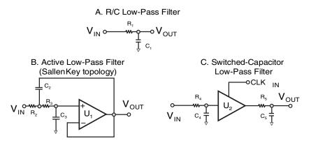
Figure 3.5: An easy low-pass filter design uses resistors and capacitors (a). The pole created by this filter is equal to  $1/(2\pi RC)$ . Multi-pole filters can use an active-filter topology (b). This  $2^{nd}$  order filter can be cascaded with more filter stages to build a higher-order filter. Switched-capacitor filters (c) are multi-pole, low-pass filters with very few external components. This type of low-pass filter can be a  $5^{th}$  (or higher) order filter.
