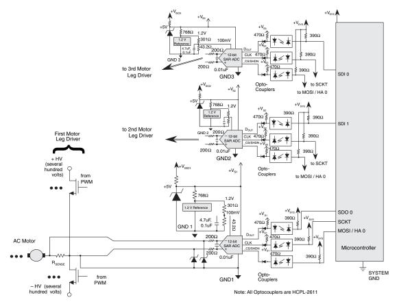
Figure 3.16: The ADC, on the isolated side of the isolation barrier, is part of the motor control sensing circuitry. The optocouplers transmit a digital signal across the barrier. Since an ADC digitizes the signal at the sensor, this circuit approach allows for better noise immunity.
