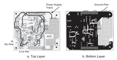
Figure 11.25: This is the layout of the top and bottom layers of the circuit in Figure 11.22. Note that this layout *does* have a ground plane.
