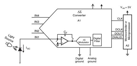
Figure 3.13: In this application circuit, the sigma-delta converter replaces the active anti-aliasing filter in Figure 3.12 with a passive R/C filter. The  $\Sigma$ - $\Delta$  converter also replaces the transimpedance amplifier (A2 and Rf). This new configuration has only two active devices plus the photosensor. In Figure 3.12, the part count is four active devices and eight passive parts.
