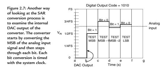
Between time (c) and (d) the analog input charge is now compared to  $\frac{3}{4}$  FS. If the MSB was found to be a "0" the MSB – 1 bit would be compared to  $\frac{1}{4}$  FS. But as you can see in this case, with the MSB equal to "1", the MSB – 1 is determined to equal "0". This process continues until the final LSB code is determined.
