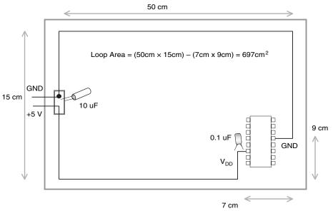
Figure 11.2: The power and ground traces are laid out using different routes to the device on this board. This mismatch opens the opportunity for EMI into the electronics of this board.
