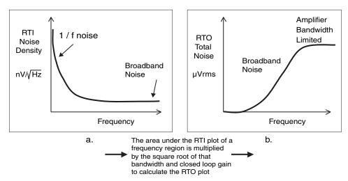
Figure 10.13: Amplifier noise can be graphically represented as if the noise source is at the input of the amplifier (a), which is otherwise known as referred-to-input (RTI), or as if it is at the output of the amplifier (b), which is otherwise known as referred-to-output (RTO).
