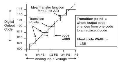
Figure A.2: The ideal transfer function has zero offset error, zero gain error, zero DNL error and zero INL error.
