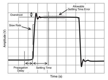
Figure 4.4: The time domain plot of a filter shows the output of the filter as it reacts to a square-wave, input signal. The key characteristics of this response are propagation delay, slew rate (SR), overshoot, settling time (ts), and settling time error ( $\varepsilon$ ).
