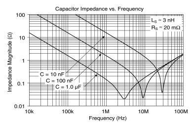
Figure 1.17: The frequency response of a capacitor varies at lower frequencies due to the series resistance and higher frequencies due to the series inductor.
