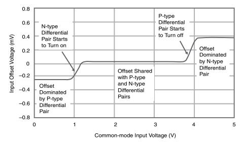
Figure 6.1: Rail-to-rail input amplifiers require two pairs of differential transistors (composite input stage, Figure 6.2c). Consequently, they have an input offset distortion as the input common-mode voltage passes through the regions where one or the other pair is turning on or off. Although the amplifier represented with this graph has two offset voltage transition regions, some single-supply, rail-to-rail input amplifiers only have one transition region.
