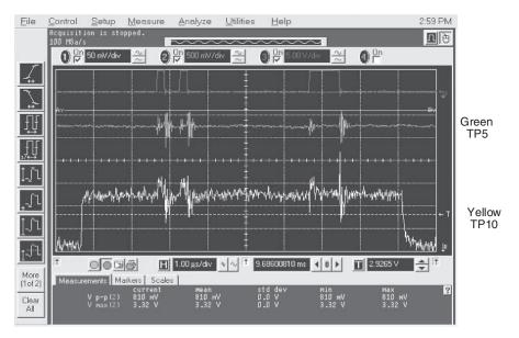
Figure 11.8: In this scope photo, the top trace was taken at JP1 (digital word to the digital potentiometers), the second trace on JP5 (noise on the adjacent analog trace), and the bottom yellow trace is taken at TP10 (noise at the output of the 16-bit DAC).
