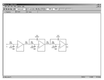
Figure 1.2: One of the views of the FilterLab program from Microchip provided analog filter circuit diagrams. This particular circuit is a 5<sup>th</sup> order, low-pass Butterworth filter with a cut-off frequency of 1 kHz. The FilterLab program from Microchip is just one example of a filter program from a semiconductor supplier. Texas Instruments, Linear Technology, and Analog Devices have similar programs available on the World Wide Web.
