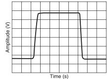
Figure 4.10: This is the step response of a 5<sup>th</sup> order, low-pass Bessel filter. As you can see in this response, there is virtually no ringing at the top or bottom of the step; only a slight time delay.
