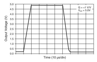
Figure 1.9: This graph illustrates the typical time domain response of the output voltage vs. time of an amplifier.
