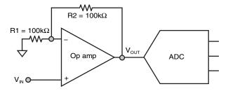
Figure 7.1: A variety of applications throughout the industry have this simple sub-circuit embedded in the system. This circuit simply takes an analog input signal and gains that signal to the output of the amplifier. For instance, an input signal of  $+1 V_{DC}$  would become a  $+2 V_{DC}$  signal at  $V_{OUT}$ . The question is, would this DC signal oscillate? Or, would a 50 kHz sinusoidal signal oscillate or ring? The bandwidth of this amplifier is 2.8 MHz.
