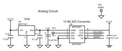
Figure 11.18: Analog section of circuit diagram for layouts in Figures 11.15, 11.16, 11.19, and 11.20. This is the circuit diagram from Microchip's MXDEV board, evaluation board for the 10- and 12-bit ADCs (MCP300X and MCP320x).
