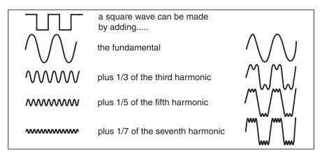
Figure B.1: You can construct a square wave using a fundamental sine wave and adding the odd harmonics of that sine wave.
