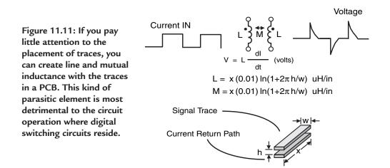
To eliminate potential noise for EMI sources it is best to separate quiet analog lines versus noisy I/O ports. Try to implement low impedance power and ground networks, minimize inductance in conductors for digital circuits and minimize capacitive coupling in analog circuits.
