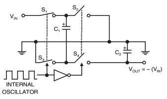
Figure 9.3: This diagram shows an ideal switched capacitor charge-pump inverter. The transfer function is  $V_{OUT} = -V_{IN}$ . You can immediately see that the input voltage is inverted, which is a nice feature if you are trying to generate a dual supply from a single-supply voltage. You will also note that the output "tracks" the input quite closely. Consequently, the output follows any variations on the input voltage, without regulation.
