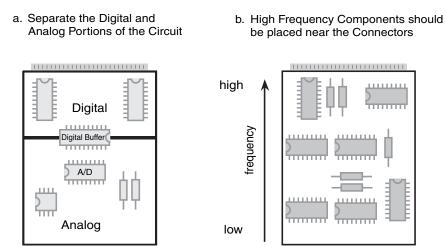
Figure 11.4: If possible, (a) the digital and analog portion of circuits should be separated in order to separate the digital switching activity from the analog circuitry. Additionally, (b) the high frequency should be separated from the low frequency where possible, keeping the higher frequency components closer to the board connector.
