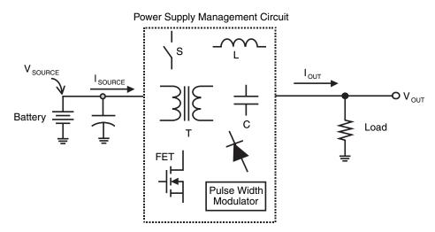
Figure 9.1: You can implement the control and reconfiguration of a power supply, such as a battery, with the three fundamental devices: SPC, charge pump or LDO. These three devices use a variety of building blocks to achieve the power-supply voltage and current transformations.
