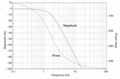
Figure 4.9: This is a 5<sup>th</sup> order, low-pass, Bessel filter response over frequency. The ratio of phase over frequency is relatively constant.
