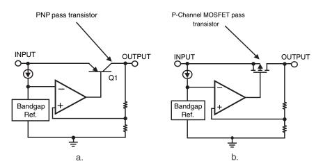
Figure 9.4: The LDO that uses a PNP pass transistor (a) sinks current from the base of the transistor to ground. Under similar conditions, the LDO that uses a P-Channel MOSFET (b) does not conduct current from the MOSFET gate to ground.
