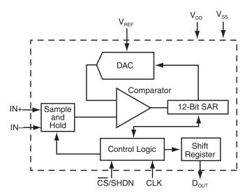
Figure 11.12: This is a block diagram of a 12-bit CMOS SAR A/D converter. This converter uses a charge distribution across a capacitive array. Refer to Chapter 2 for more information on how these devices actually work.
