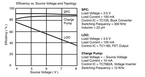
Figure 9.5: This graph shows the difference of the efficiency versus input voltage of SPC, LDO, and charge pump circuits. It illustrates that an SPC device is the most efficient device, when the source voltage is dynamic. The LDO device is the least efficient circuit in a system, showing a decreasing linear relationship of efficiency with respect to the source voltage.
