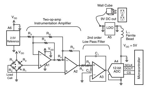
Figure 10.5: This modified circuit is basically the same as the circuit in Figure 10.3. The modifications include the addition of a low-pass, anti-aliasing filter, bypass capacitors and an inductive ferrite bead ( $L_1$ ) on the power supply trace.
