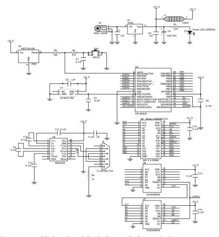
Figure 11.17: Digital section of circuit diagram for layouts in Figures 11.15, 11.16, 11.19 and 11.20. This is the circuit diagram from Microchip's MXDEV<sup>™</sup> board, evaluation board for the 10- and 12-bit ADCs (MCP300X and MCP320x).
