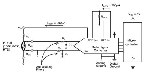
Figure 3.8: A  $\Sigma$ - $\Delta$  ADC directly digitizes the small signal from a four-terminal, RTD temperature sensor. In this circuit, a 200  $\mu$ A current reference from the  $\Sigma$ - $\Delta$  ADC excites the temperature sensor. The 200  $\mu$ A current source is ratiometric to the ADC voltage reference. The resistor/capacitive pairs (R1/C1) are used as anti-aliasing, low-pass filters.
