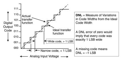
Figure A.3: The differential nonlinearity is the difference between an ideal code width and the measured code width.
