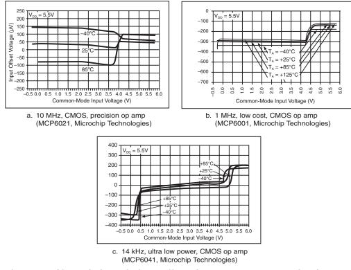
Figure 6.3: This graph shows the input-offset voltage versus common-mode voltage of three different CMOS operational amplifiers over temperature with a single-supply voltage of 5.5 V. All three amplifiers have rail-to-rail input swing capability.
