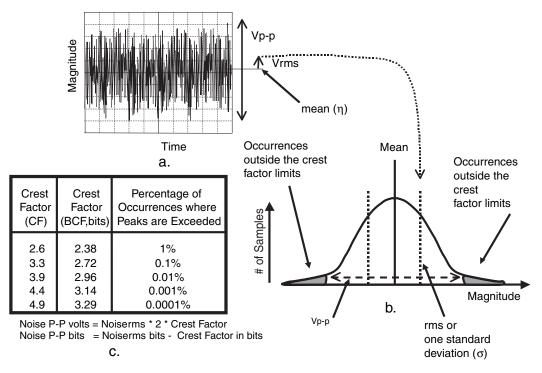
Figure 10.2: If noise is a random event (a), these "obviously" unpredictable events can be characterized with a normal distribution (b) where you can calculate mathematical equivalents of the mean ( $\eta$ ) and standard deviation ( $\sigma$ ). If you multiply the standard deviation (equal to rms by a 2x crest factor, you can predict the probability of occurrences outside the crest factor limits (b and c).
