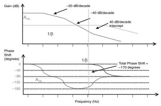
Figure 6.23: In a practical circuit implementation, given layout parasitics, this system is also unstable.
