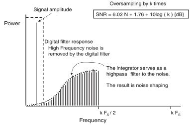
Figure 2.16: The noise in the modulator is moved out into higher frequencies. This is called noise shaping. After the modulator, the digital filter is used to implement a low-pass filter where high-frequency noise is removed. The calculation for the SNR includes the effects of oversampling.
