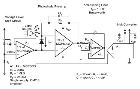
Figure 6.10: In photo detection circuits, the amplifier input bias current could generate voltage drop across the parallel combination of  $R_F$  and the photodiode parasitic resistance. In anti-aliasing filter circuits, input bias current can generate a voltage error across input resistors ( $R_s$  and  $R_6$ ).
