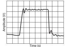
Figure 4.8: This is the step response of a 0.5 dB, low-pass, 5<sup>th</sup> order Chebyshev filter. With this filter the ringing is longer lasting than you will find with the Butterworth or Bessel filter.
