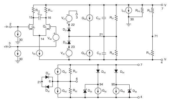
Figure 7.7: This is an example of a SPICE macromodel for a CMOS input amplifier. In this circuit, the SPICE simulation generates an input bias current error as an artifact of the SPICE constraints. Alexander and Bowers were the first to go public with this macromodel. This information appeared in the Electronic Design Magazine in 1990.
