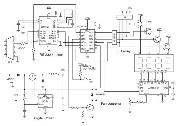
Figure 13.8: This is the circuit implementation of the digital portion of the block diagram in Figure 13.5. This circuit includes the microcontroller, RS-232 interface, LED array, fan controller and digital power.
