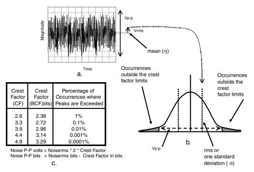
Figure 2.5: A sample of an ADC's output can be collected in time (a) and translated into a histogram (b) where the mean and standard deviation of the samples can be calculated. With the standard deviation of these samples, a peak-to-peak value can be determined (c) with a multiple of 2 times the crest factor (CF) for output signal referred to input calculations or an additive bit crest factor (BCF).
