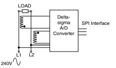
Figure 1.6: A power meter application requires <12-bit resolution in the system. This may imply that a simple 12-bit SAR converter can do the job, but the required LSB size is much smaller than the SAR converter can provide. Consequently, a sigma-delta converter is often used.
