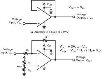
b. Amplifier in a Gain of -1V/V
