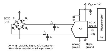
Figure 3.11: The voltage at the output of the SCX015 pressure sensor is filtered at both inputs to the sigma-delta ADC by single-pole low-pass filters (R1/C1) and digitized by the sigma-delta ADC (A4).
