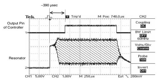
Figure 9.11: The start-up time of a 4 MHz resonator is faster than a 4 MHz crystal and slower than a 4 MHz internal clock.
