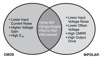
Figure 5.2: The two silicon technologies that single-supply amplifiers are manufactured with are CMOS or bipolar processes. By using the CMOS process, you can manufacture bipolar amplifiers. In these designs, the input transistors are bipolar, and the remaining transistors are CMOS.
