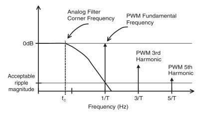
Figure 8.4 show a simplified FFT plot of the signal in Figure 8.1.
