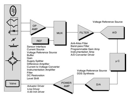
Figure 1.19: This signal chain is somewhat universal in that it deals with the analog signal coming in, conditions it through the amplification system and digitizes it in preparation for the microcontroller or processor.
