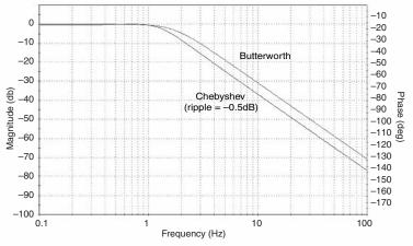
Figure 4.18: Of the Butterworth and Chebyshev designs, the Chebyshev exhibits the fastest roll-off over frequency after the cut-off frequency of the filter. Since this is a DC application, the Chebyshev is the best candidate.
