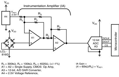
Figure 1.10: The circuit in this diagram uses a 12-bit A/D converter in combination with an instrumentation amplifier to convert the low-signal, output of a Wheatstone bridge sensor to usable digital codes.
