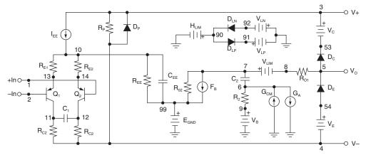
Figure 7.10: This PNP operational amplifier macromodel was originally designed in 1974 by Graeme R. Boyle, Barry M. Cohn, Donald O. Pederson, James E. Solomon. It was the first legitimate model published. Several other operational amplifier macromodel templates have been developed since then. Some SPICE vendors provide tools in their software to generate this type of macromodel.
