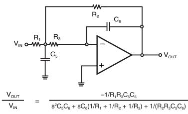
Figure 4.16: A double-pole, multiple feedback circuit implementation uses three resistors and two capacitors to implement a  $2^{nd}$  order analog filter. DC gain is equal to  $-R_2/R_1$ .
