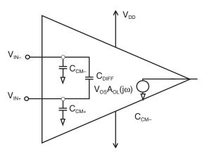
The two input terminals have common-mode capacitances to ground ( $C_{CM}$ ) and differential capacitance ( $C_{DIFF}$ ) between the inputs.  $A_{OL}(j\omega)$  represents the open-loop gain, frequency response of the amplifier. Figure 6.16 shows the frequency response of a typical voltage feedback amplifier using the Bode plot method.
