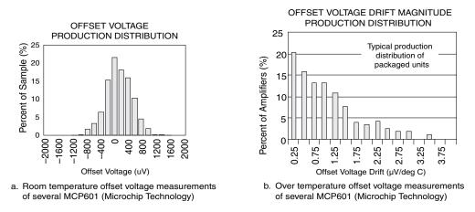
Figure 6.12: The offset voltage of several devices from a production run (a) can vary from device to device. The same is true for the offset voltage change over temperature (b).
