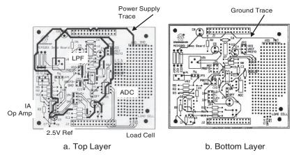
Figure 11.23: This is the layout of the top (a) and bottom (b) layers of the circuit in Figure 11.22. Note that this layout does not have a ground or power plane. Note that the power traces are considerably wider than the signal traces in order to reduce power supply trace inductance.
