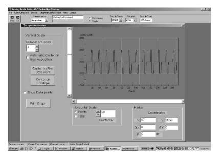
Figure 12.7: The time domain representation of this data from the 12-bit A/D converter produces an interesting periodic signal. This signal was traced back to the power supply. Each graph in Figure 12.5, 12.6, and 12.7 uses the same data.
