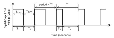
\*The fundamental frequency of PWM signal = 1/T
