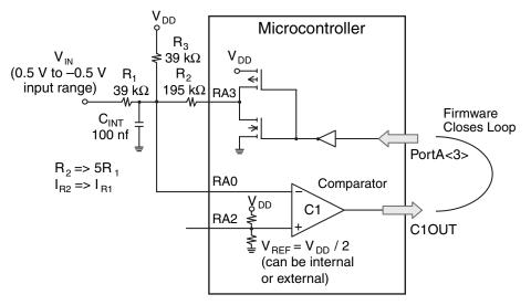
Figure 8.18: Configuration of the microcontroller for a sigma-delta conversion with a +/-500 mV range centered around ground.
