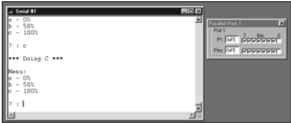
FIGURE 33.8 Illustrating the use of the example 3-level PWM library in the Keil hardware simulator
