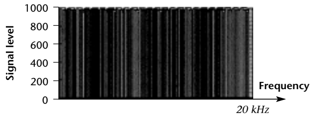
FIGURE 32.18 The representation of a broadband signal (bandwidth 20 kHz) in the frequency domain
