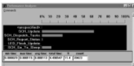
FIGURE 14.6 Using the Keil hardware simulator to evaluate the CPU load imposed by a scheduler with 1 ms ticks, running on a 12 MHz (12 oscillations per instruction) 8051 11% idle.
