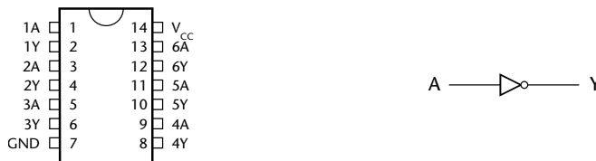
FIGURE 7.9 Pinout of the 74x04 inverter and corresponding logic diagram (positive logic). (Reproduced courtesy of Texas Instruments)
