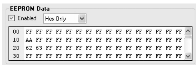
(d) PICkit2 verification of the three writes
